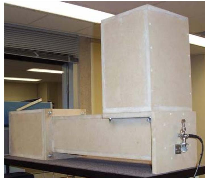
Figure 2: Acoustic duct environment
