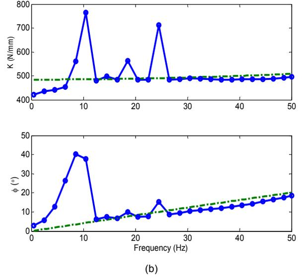
Fig. 7  $\tilde{K}(f, X)$  results of a free decoupler mount with (a)  $X = 0.3$  mm and (b)  $X = 0.5$  mm. Key: — measured spectra, --- curve-fit result using the Voigt visco-elastic model.
