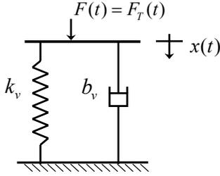
Fig. 6 Voigt visco-elastic model at lower  $f$  when the inertia track is completely decoupled.
