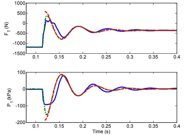
Fig. 9 Step responses for a fixed decoupler mount. Key: — Measurement given excitation of Fig. 8, - - - Numerical simulation based on the quasi-linear model (with  $X = 1.5$  mm and excitation of Fig. 8), - - - Analytical solution assuming an ideal step input [14].
