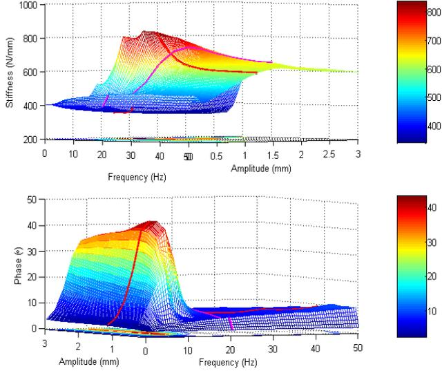
Fig. 1 Surface interpolated  $\tilde{K}(f, X)$  data from discrete stiffness measurements
