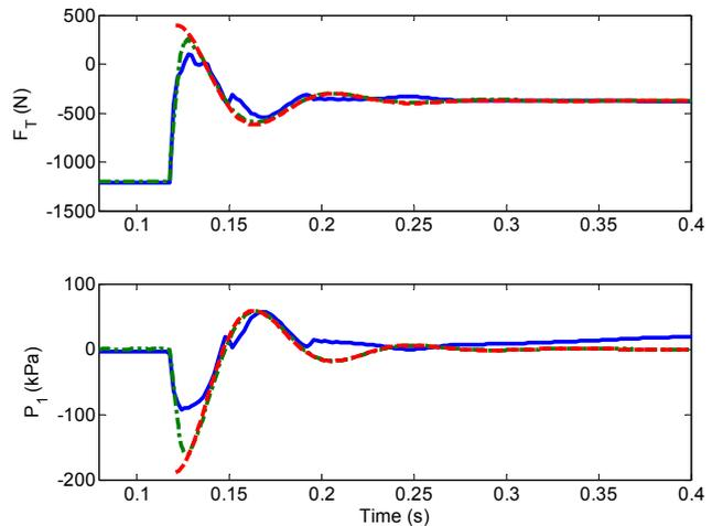
Fig. 10 Step responses for a free decoupler mount. Key: — Measurement given excitation of Fig. 8, - - - Numerical simulation based on quasi-linear model (with  $X = 2$  mm and given excitation of Fig. 8), - - - Analytical solution assuming an ideal step input [14].
