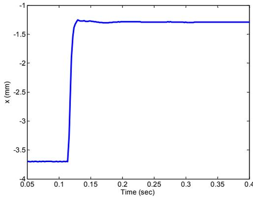
Fig. 8 Measured step-like displacement excitation  $x(t)$  from -3.7 to -1.32 mm.
