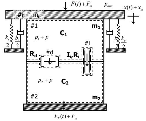
Fig. 2 Lumped fluid model of a generic hydraulic engine mount
