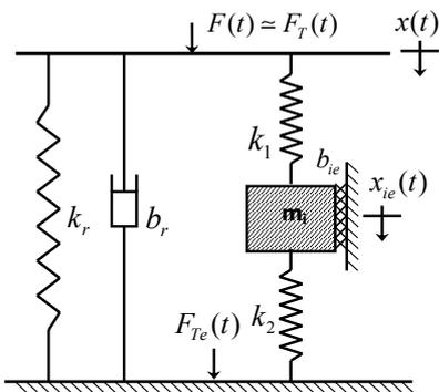
Fig. 3 Analogous mechanical system for a fixed decoupler mount assuming a dynamic force excitation  $F(t)$ .
