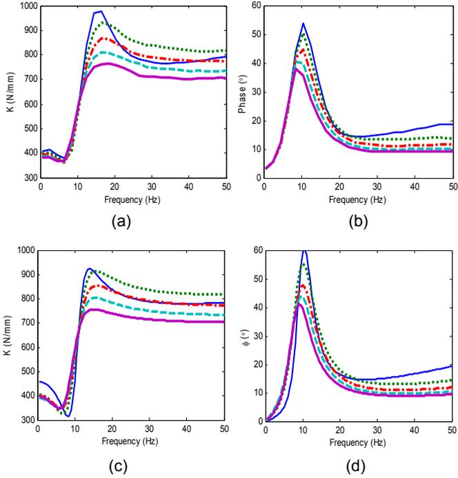
Fig. 5 Dynamic stiffness of a free decoupler mount. Measurements are in (a), (c); and (b), (d) show  $K_{32}$  predictions. Key: From top to bottom (p-p):  $X = 1.0, 1.5, 2, 2.5, 3$  mm.
