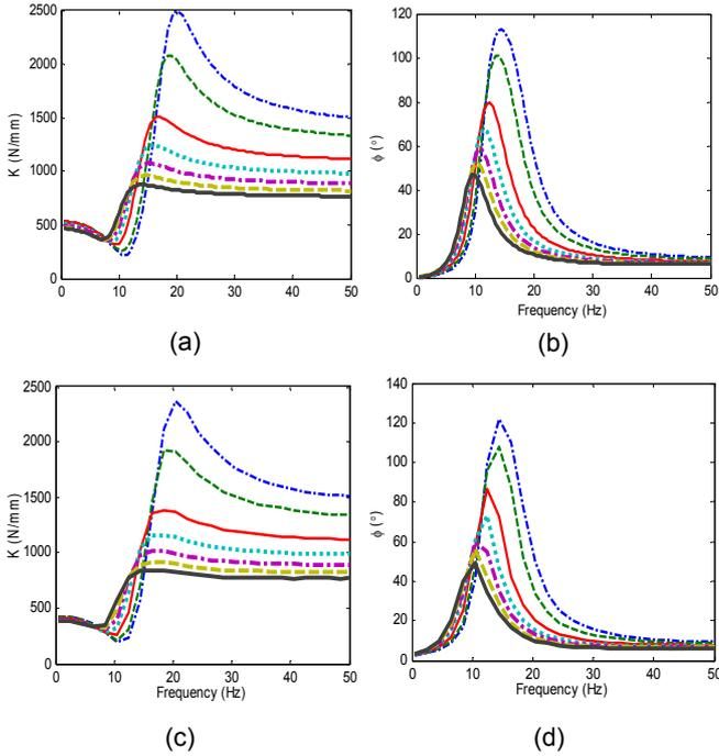
Fig. 4 Dynamic stiffness of a fixed decoupler mount. Measurements are in (a), (c); and (b), (d) show  $K_{32}$  predictions. Key: From top to bottom (p-p)  $X = 0.3, 0.5, 1.0, 1.5, 2, 2.5, 3 \text{ mm}$ .
