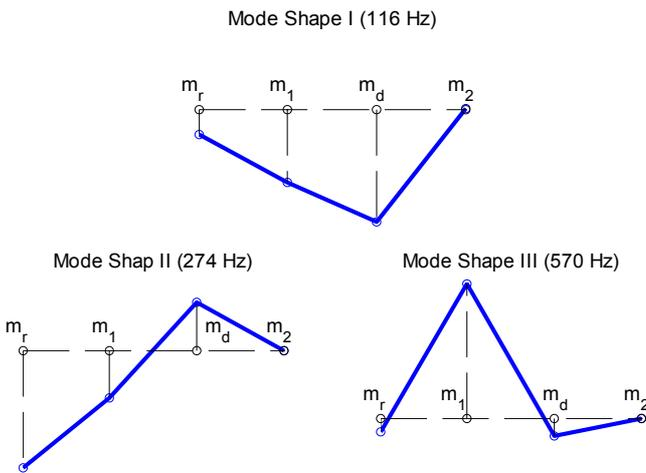
Fig. 13 Displacement mode shapes of the 3DOF model considering the effect of a bell plate in the upper chamber (a design suggested by Geisberger *et al.* [6]).
