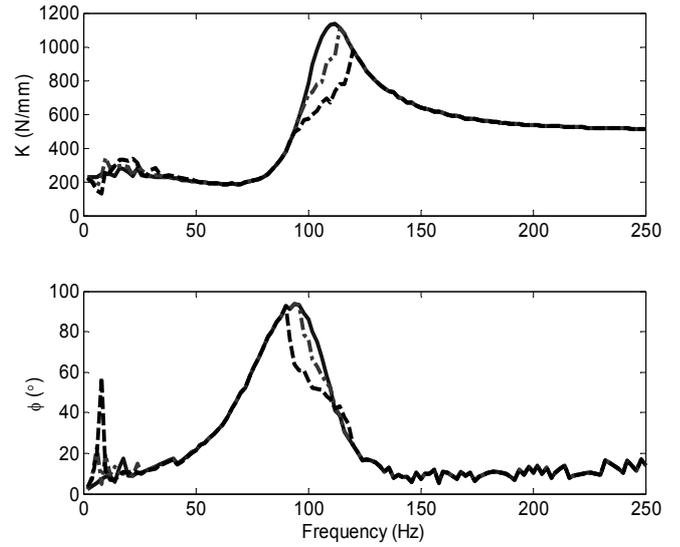
Fig. 20 Predicted dynamic stiffness over the higher frequency regime using Model I [7,8]. Key: —  $X = 0.05$  mm, .....  $X = 0.075$  mm; - - -  $X = 0.1$  mm
