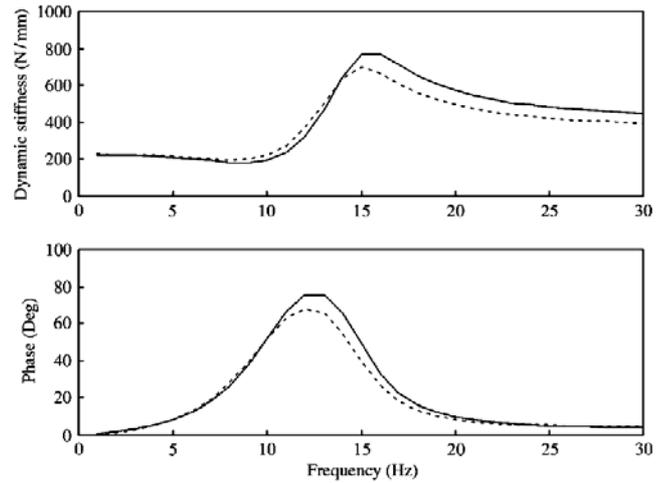
Fig. 22 Prediction using Model II over the lower frequency regime [12]. Key: —  $X = 2$  mm; - -  $X = 1$  mm.
