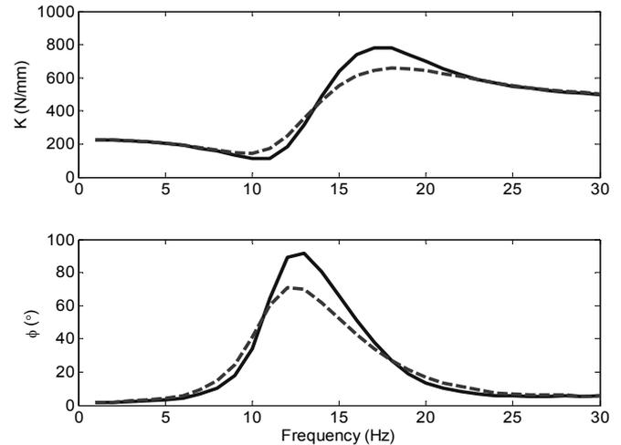
Fig. 23 Prediction using Model I over the lower frequency regime. Key: —  $X = 2$  mm; - -  $X = 1$  mm.
