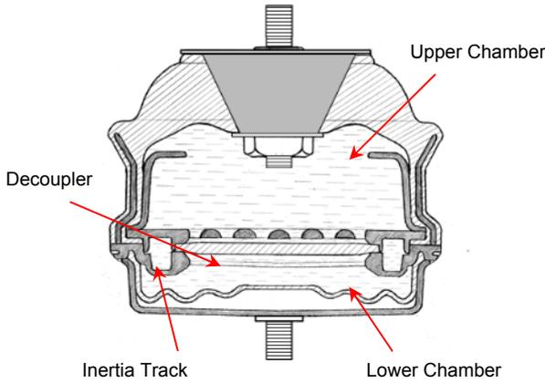
Fig. 1 Schematic of free decoupler mount G.
