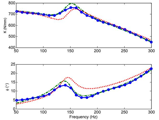
Fig. 16 Dynamic stiffness of mount G with  $X = 0.1$  mm. Key:  $\bullet$  measurement,  $---$   $4^{th}/2^{nd}$  curve-fit,  $\cdots$  predicted using the  $4^{th}/2^{nd}$  mechanical model.
