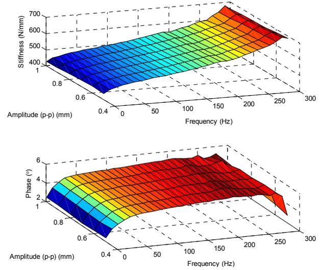
Fig. 6 Measured dynamic stiffness of the rubber element of mount G up to 300 Hz, given  $X = 0.5 \sim 1$  mm (p-p).
