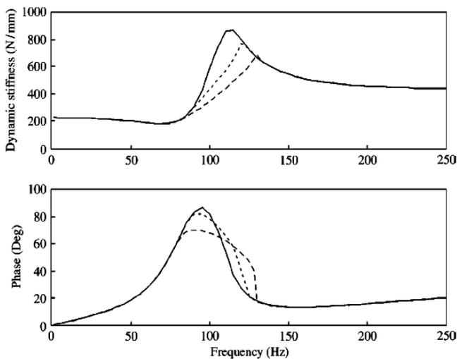
Fig. 19 Predicted dynamic stiffness over the higher frequency regime using Model II [12]. Key: —  $X = 0.05$  mm, .....  $X = 0.075$  mm; - - -  $X = 0.1$  mm.
