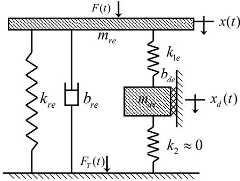
Fig. 15 Simplified 2DOF high frequency mechanical model.
