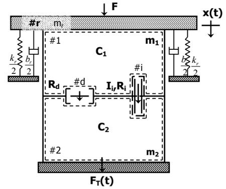
Fig. 17 Model I: Nonlinear fluid model of a free decoupler mount [7, 8].
