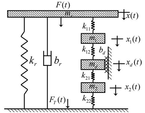
Fig. 4 A simplified mechanical model with 4DOF proposed to describe the higher frequency dynamics.
