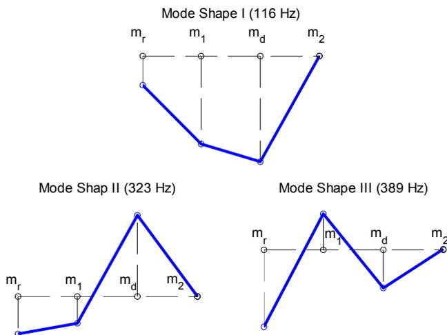
Fig. 9 Displacement mode shapes of the 3DOF mechanical model of Fig. 5.
