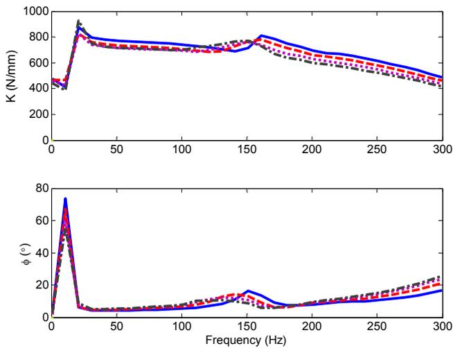
Fig. 8 Measured dynamic stiffness of mount G up to 300 Hz.
