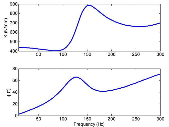
Fig. 7 Predicted dynamic stiffness of mount G using linear 3DOF model of Fig. 4.
