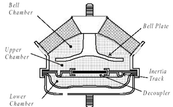
Fig.10 Cross section of mount Q with a bell plate in the upper chamber; extracted from Geisberger *et al.* [6].
