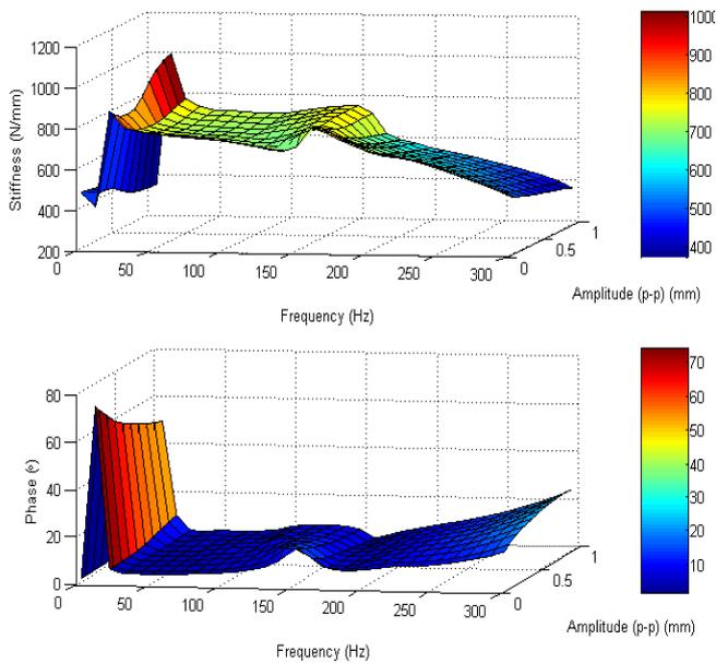
Fig. 2 Measured dynamic stiffness of mount G up to 300 Hz.
