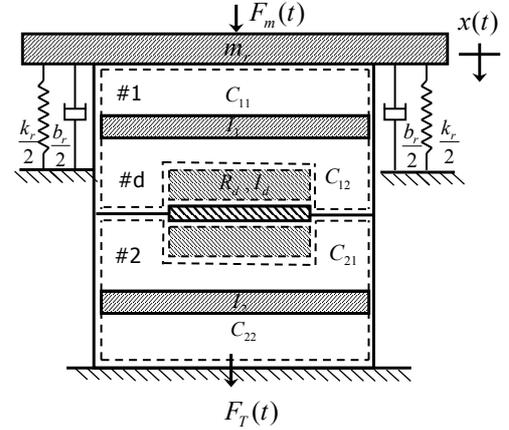
Fig. 3 Schematic of the lumped fluid model.
