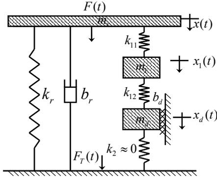
Fig. 5 Reduced order mechanical model (3DOF) over the higher frequencies.
