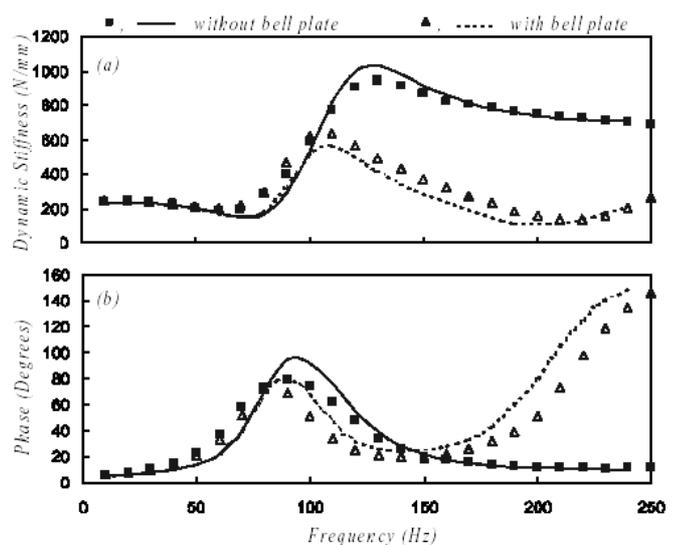
Fig. 11 Dynamic stiffness of mount Q with  $X = 0.1$ mm. Results are extracted from Geisberger *et al.* [6]. Key: “■, —” without and “▲, - - -” with bell plate structure.
