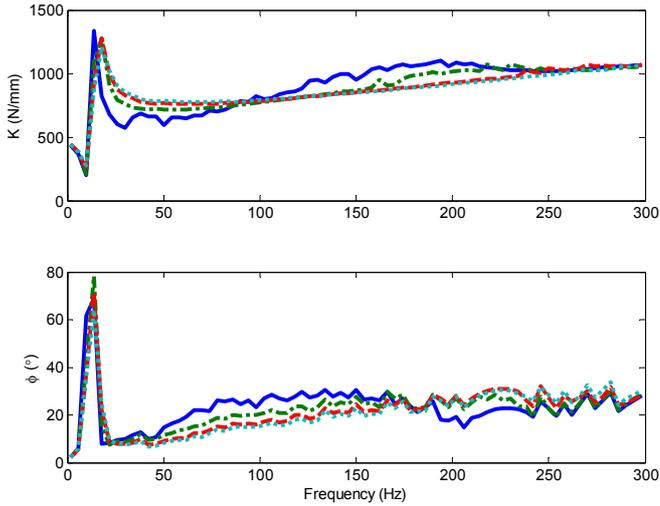
Fig. 21 Predicted dynamic stiffness of mount G using nonlinear model I. Key: —  $X = 0.1$  mm, - -  $X = 0.2$  mm, ····  $X = 0.4$  mm, - · - ·  $X = 0.6$  mm.
