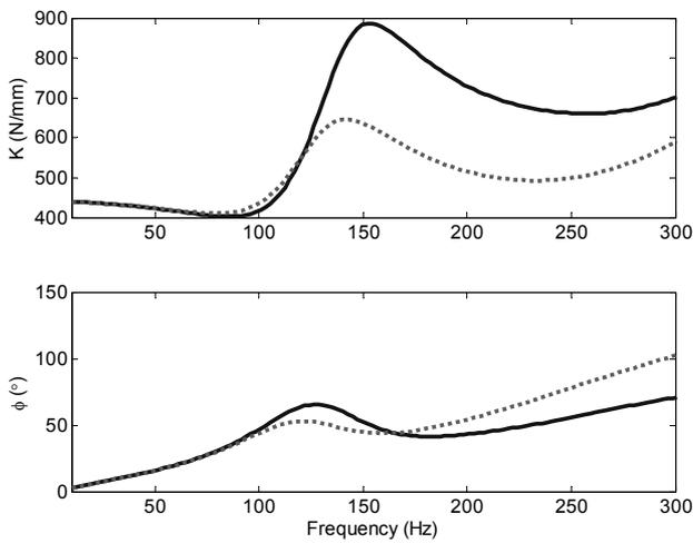
Fig. 12 Predicted dynamic stiffness of mount G using 3DOF model. Key: “—” original (without bell plate), “...” with a bell plate. Corresponding experimental results are in Fig. 11.
