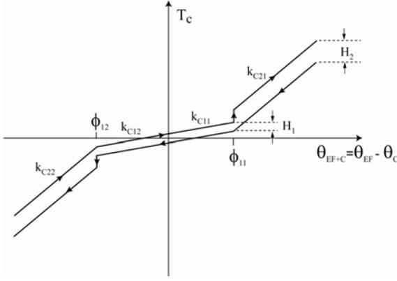
Figure 4 Non-linear characteristics of a dual-staged clutch damper.
