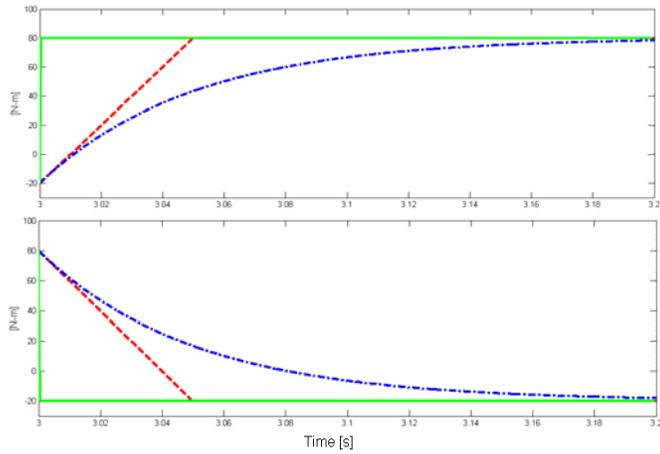
Figure 9 Simplified engine torque shapes  $T_{ENG}(t)$  for tip-in and tip-out events. Key: — Torque A - - - Torque B - · - Torque C.
