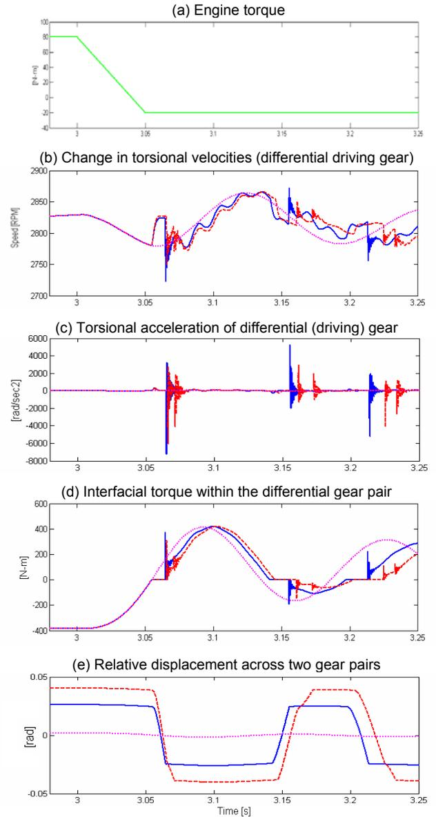
Figure 10 Comparison of impulsive behavior between zero, one, and two backlash elements during the tip-out event. Key: — One Backlash - - - Two Backlashes ····· Zero Backlash
