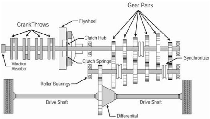
Figure 1 Example case: 4x2 front wheel drive system with manual transmission.
