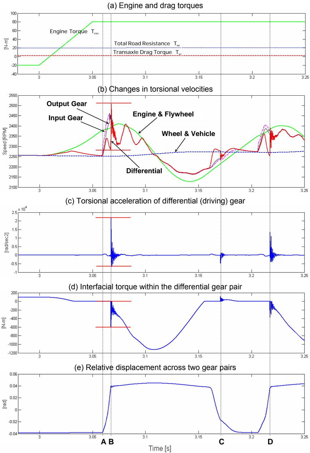
Figure 7 Clunk events in the non-linear model of Figure 3 with a dual clutch damper during the tip-in event
