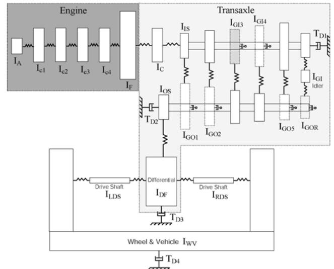
Figure 2 Linear torsional model of the example case: 19-DOF undamped system in the 3<sup>rd</sup> engaged gear.
