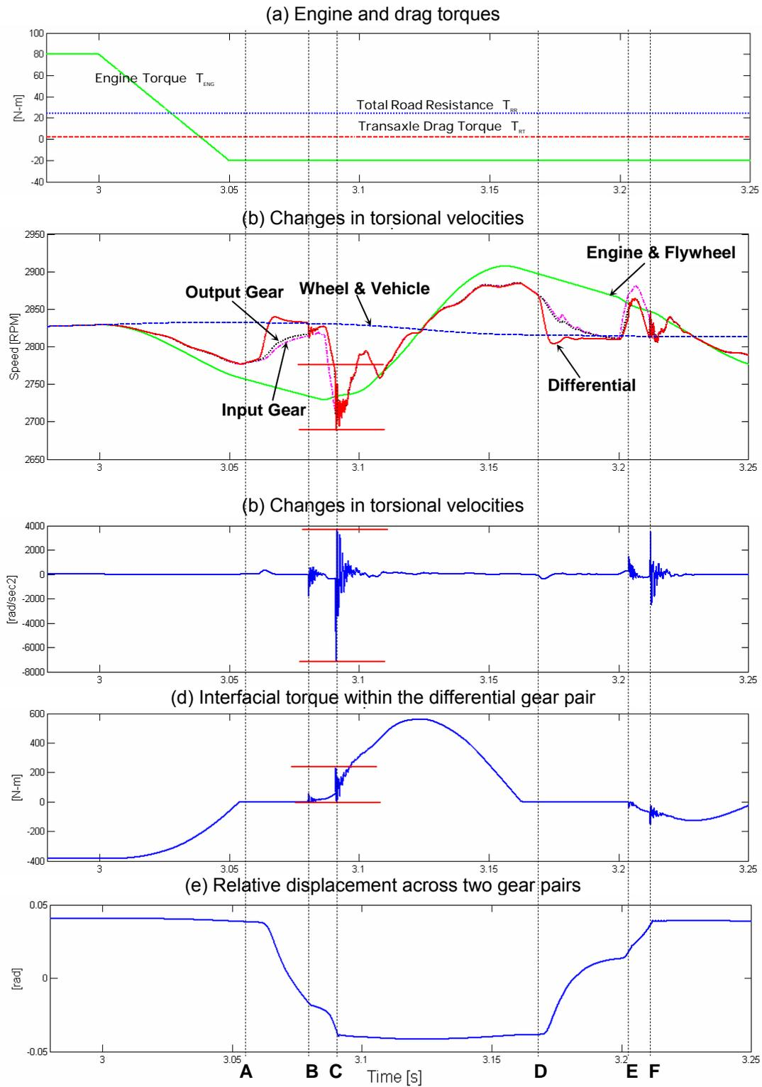
Figure 8 Clunk events in the non-linear model of Figure 3 with a dual clutch damper during the tip-out event
