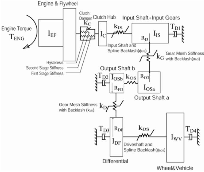
Figure 3 Non-linear torsional model of the example case in the 3<sup>rd</sup> engaged gear: 7-DOF system with a multi-staged clutch damper and multiple gear pairs and hub-spline interfaces with backlashes.
