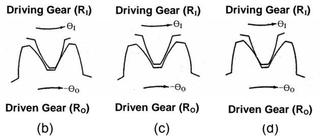
Figure 6 Inclusion of backlash in gear mesh forces or spline interface torques. (a) Non-dimensional non-linear function (b) gears are in contact on the driving side ( $x_r > x_b$ ) (c) gears are separated in the backlash regime ( $-x_b < x_r < x_b$ ) and (d) gears are in contact on the driven side ( $x_r < x_b$ ). Here  $x_r = R_i\theta_i + R_o\theta_o$  and  $x_b$  corresponds to  $b$  in (a).
