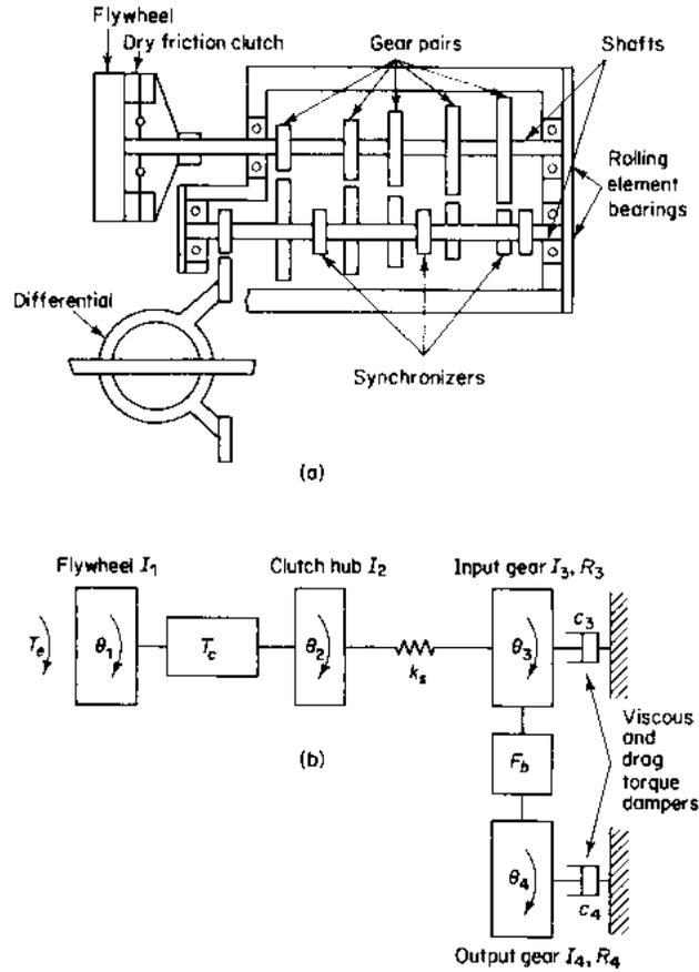
**Figure 11:** Physical model for the neutral gear rattle problem. (a) Automotive manual transmission schematic; (b) a simplified torsional model.
