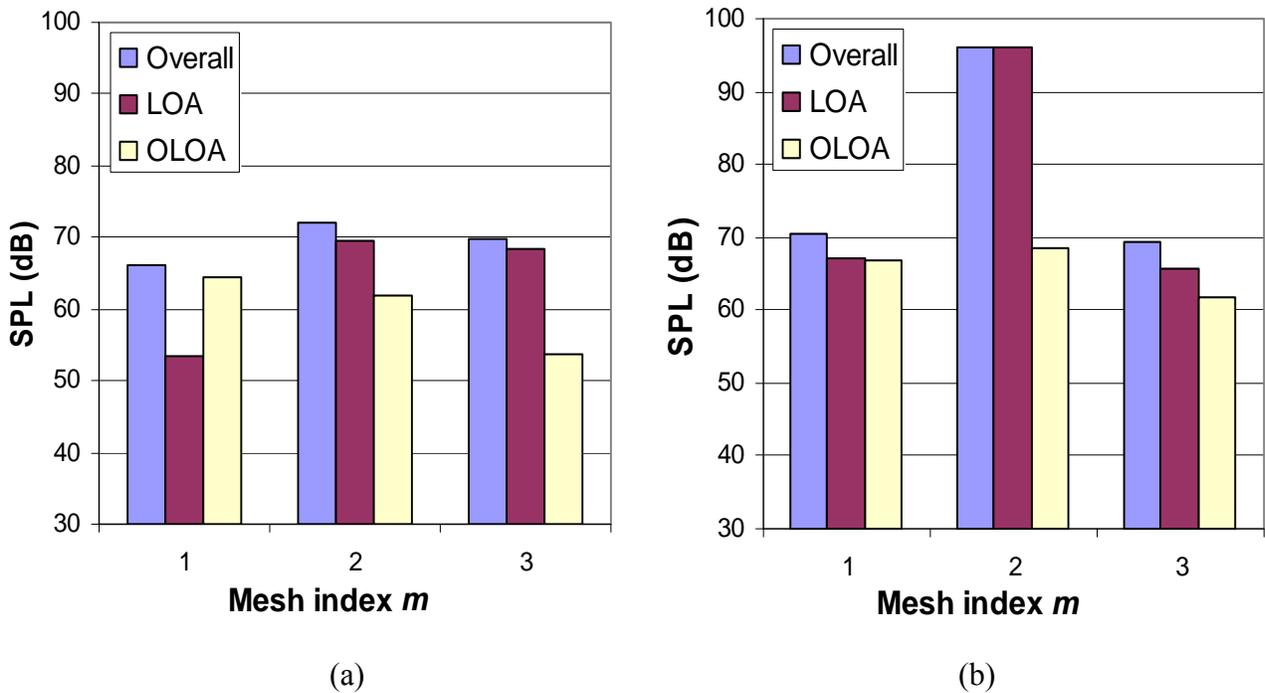
**Figure 10:** Overall sound pressure levels (dB re 2e-5 Pa) and their contributions predicted at 6" above the top plate under  $\Omega_p = 4875$  RPM and 140 °F. (a) Mean load  $T_p = 500$  lb-in (optimal load for minimum transmission error); (b) mean load  $T_p = 800$  lb-in. Key: LOA = line-of-action; OLOA = off-line-of-action.
