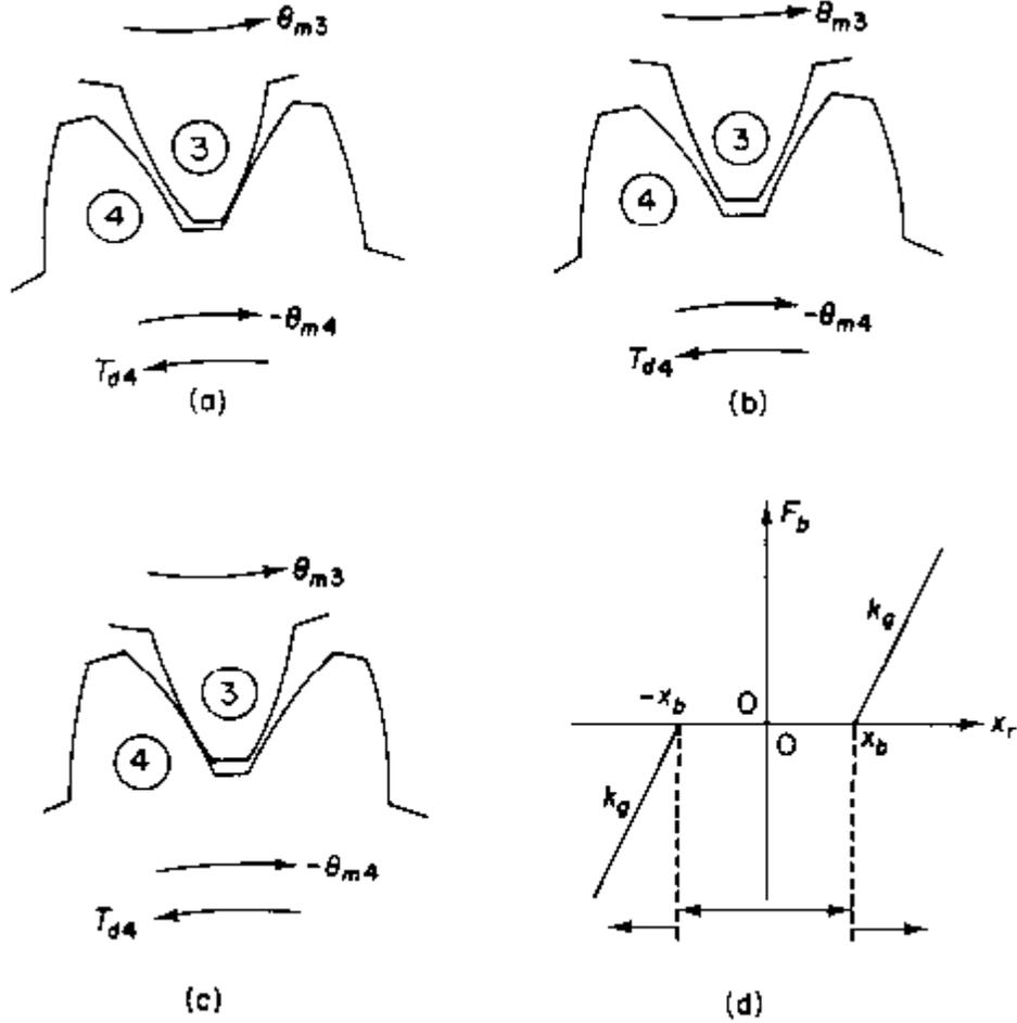
**Figure 13:** Meshing gears and gear mesh force  $F_b$ . (a) Gears in contact on the driving side; (b) gears separated; (c) gears in contact on the driven side; (d) elastic compression force ( $F_b$ ) with gear teeth meshing stiffness ( $k_g$ ) and backlash ( $2x_b$ ). Here, the relative displacement is  $x_r(t) = R_3\theta_3 + R_4\theta_4$ .
