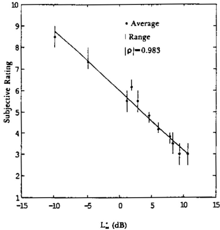
**Figure 2:** Subjective ranking versus perceived gear whine level  $L_{ms}^* = 10 \text{Log}_{10} E_{ms}^*$  (in dB) obtained from spatially averaged microphone ( $L_p$ ) and accelerometer signals ( $L_{a1}$  and  $L_{a2}$ ) with  $m = 3$ , bandwidth ( $B_m$ ) ranging from 10 to 70 Hz and correlation coefficient  $|\rho| = 0.983$ .
