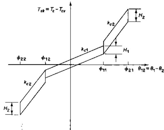
**Figure 12:** Dynamic characteristics of a simplified clutch damper. Here  $T_{cv} = c_{12}\dot{\theta}_{12}$  is the viscous damping torque,  $k$  is the stiffness, and  $H$  is the hysteresis. This curve is asymmetrical in operational angles ( $\phi$ ); i.e.  $\phi_{11} \neq \phi_{12}$  and  $\phi_{21} \neq \phi_{22}$ . See Singh et al. (1989) for details.
