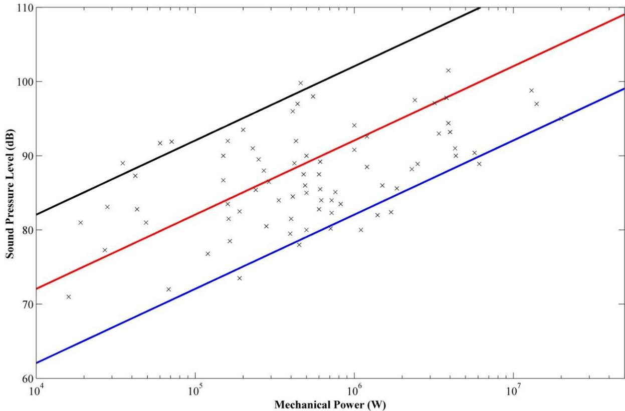
**Figure 1:** Influence of mechanical power transmitted ( $W_{\text{mech}}$ ) and acoustic efficiency ( $\eta_a$ ) on the overall gear (whine) noise levels in terms of  $L_p$  (dB re  $20 \mu\text{Pa}$ ) at  $r = 4 \text{ m}$ . Key: x measured noise data reported by Optiz (1968); — (black) Eq. (1) with  $\eta_a = 2 \times 10^{-6}$ ; — (red) with  $\eta_a = 2 \times 10^{-7}$ ; — (blue) with  $\eta_a = 2 \times 10^{-8}$ .
