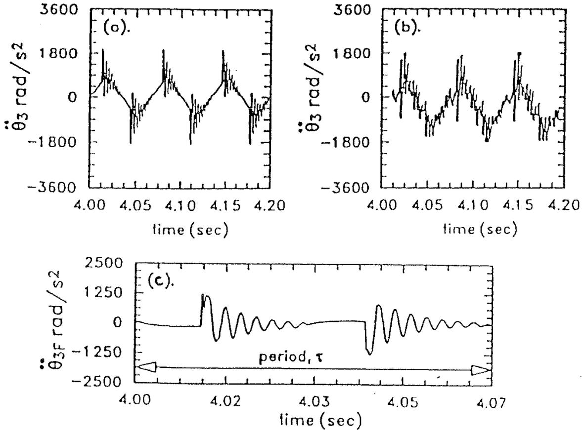
**Figure 15:** Typical gear rattle signatures in terms of angular acceleration time histories obtained from a. computer simulation, b. experimental measurements, and c. filtered signal shown in a.
