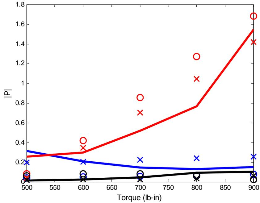
**Figure 9:** Sound pressures (Pa) at the first three gear mesh frequencies (with speed  $\Omega_p = 4875$  RPM) over a range of torque  $T_p$  at 140 °F. Key: —, measurements (6" above the top plate); ○, Rayleigh integral predictions; ×, substitute source predictions. Color code: Blue, gear mesh frequency harmonic  $m = 1$ ; red,  $m = 2$ ; black,  $m = 3$ . Note that this formulation utilizes analytical descriptions of sources, paths, and radiators.
