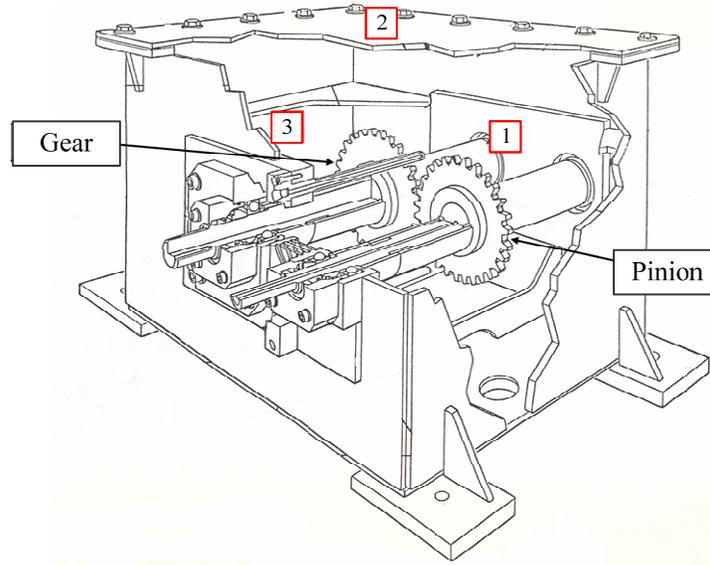
**Figure 7:** Schematic of the NASA spur gearbox.
