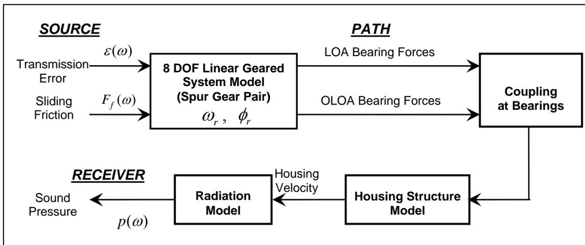
**Figure 3:** Conceptual description of the vibro-acoustics of a geared system with two excitations, given linear system assumption
