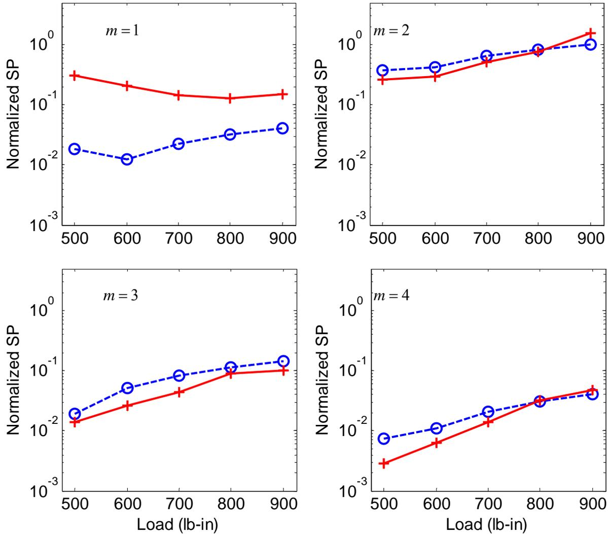
**Figure 5:** Comparison of the normalized sound pressure (SP) predictions with measurements at the first four gear mesh harmonics ( $m = 1, 2, 3, 4$ ). Key:  $+$ , measurements;  $-o-$  predictions. Note that this formulation utilizes empirical structural path and receiver models.
