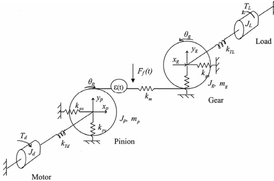
**Figure 4:** Schematic of the whine source (8 DOF geared system) model with two gear noise sources for a spur gear pair (damping elements not shown)
