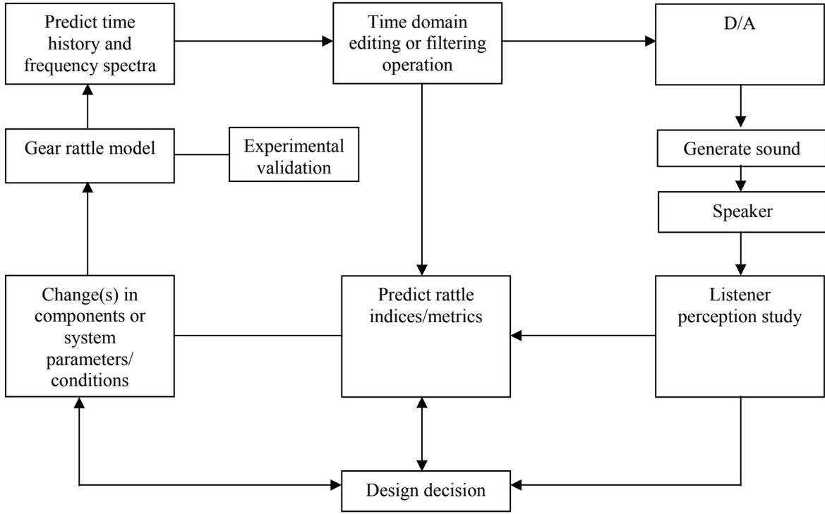
**Figure 14:** Flowchart of gear rattle simulation post-processing stage
