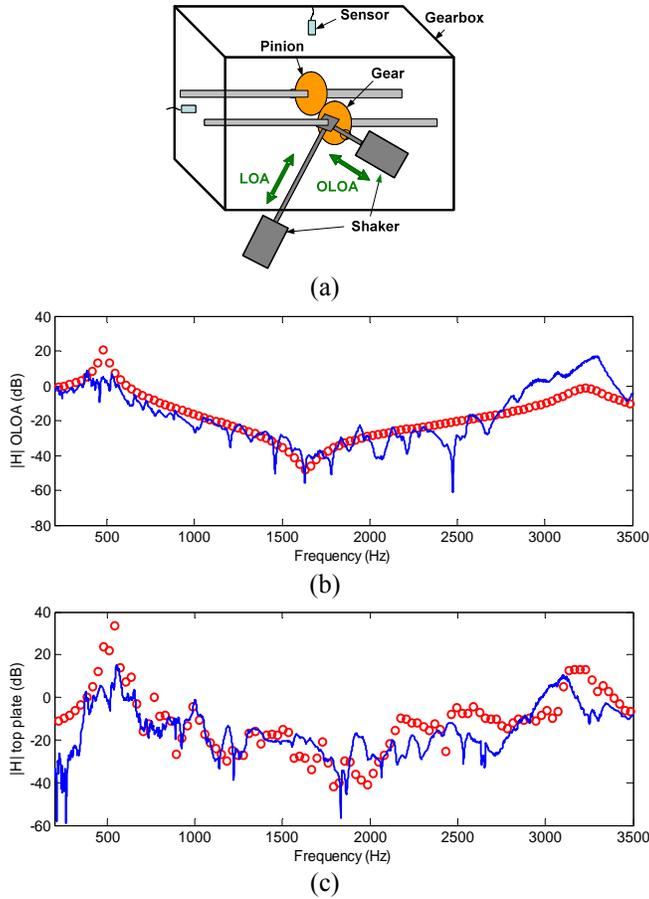
**Figure 8:** (a) Experiment used to measure the structural transfer functions; (b) Comparison of the transfer function magnitudes from gear mesh to bearings; (c) Comparison of the transfer function magnitudes from gear mesh to a sensor on the top plate (gearbox). Key:  $\circ$ , measurements; — predictions.
