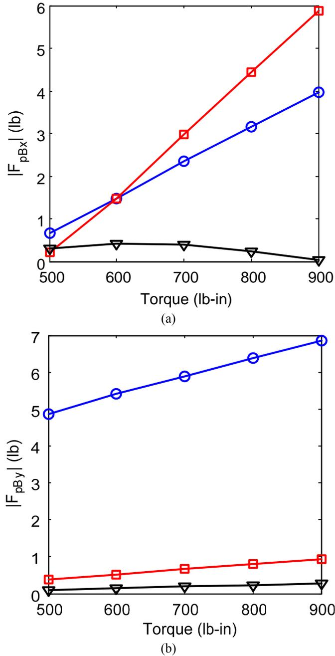
**Figure 6:** Dynamic bearing forces predicted over a range of  $T_p$  given  $\Omega_p = 4875$  RPM and  $140$  °F. (a): Line-of-action (LOA) bearing force in the x direction; (b) off-line-of-action (OLOA) bearing force in the y direction. Key:  $m$  is the gear mesh frequency harmonic. Key:  $\text{---}\circ\text{---}$ ,  $m = 1$ ;  $\text{---}\square\text{---}$ ,  $m = 2$ ;  $\text{---}\nabla\text{---}$ ,  $m = 3$ .
