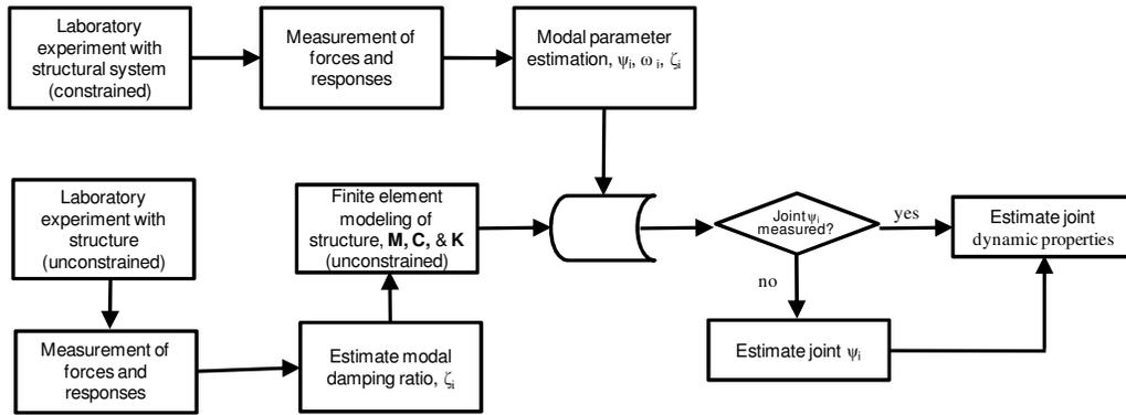
**Fig.2** Flow-chart of the inverse joint identification method. Refer to Noll, et al. [8] for mathematical details.
