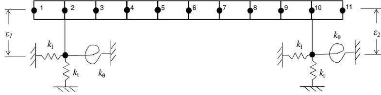
**Fig. 3** Computational beam model with 10 elements and 11 nodes. Lumped stiffness elements are attached at nodes 2 and 10.
