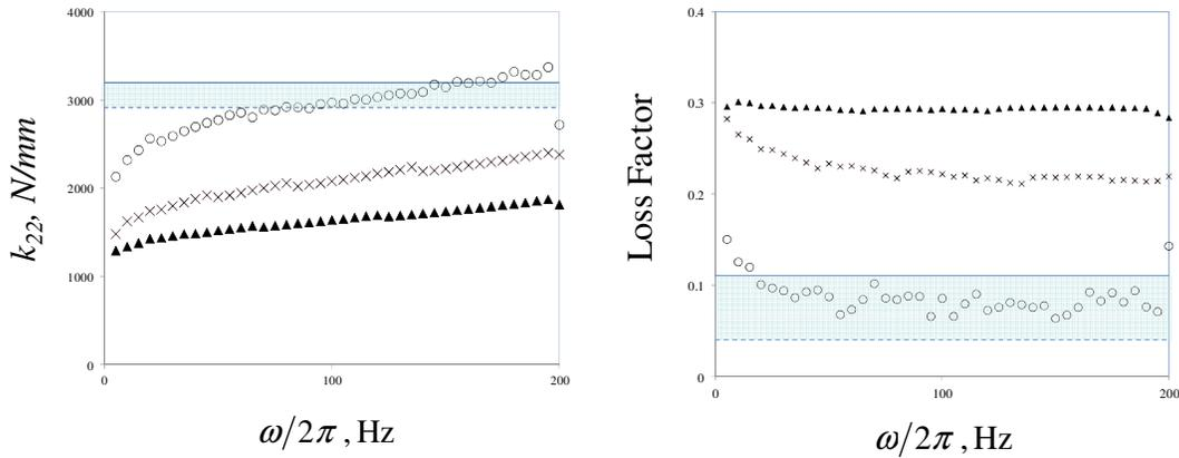
**Fig. 6** Comparison of stiffness and loss factor identified through inverse and direct tests. key: direct test with pk-pk amplitude of  $\circ$  0.01mm,  $\times$  0.05 mm, and  $\blacktriangle$  0.1 mm ;  $\text{shaded region}$  inverse method with 95% confidence interval.
