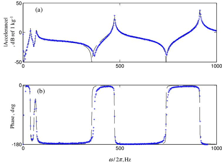
**Fig. 4** Driving point acceleration for the resonant beam experiment in the transverse direction at point 3 as displayed in Fig. 3: (a) magnitude; (b) phase. Key: (—) predicted using Eqn. (2) ; (+) measured.
