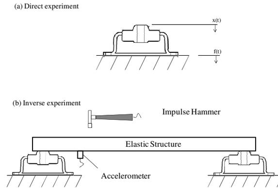
**Fig. 1** Schematic of the direct and inverse experiments: (a) elastomeric mount loaded in compression and excited by a displacement input; (b) elastic beam is end supported by two mounts, where each is bolted to the beam; it is excited by an impulse hammer.
