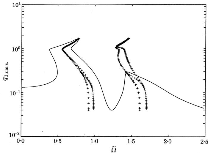
Figure 11. The frequency response of the system, showing the dependence of the natural frequencies on the response amplitude, given  $b_1 = 1.00$ ,  $b_2 = 0.10$ ,  $Q_{m,1} = Q_{m,2} = 0.50$ ,  $Q_{a,1} = 0.25$ ,  $Q_{a,2} = 0.00$  and  $\Delta\omega^* = 0.73$ . —, Response characteristics; +, backbone curve.
