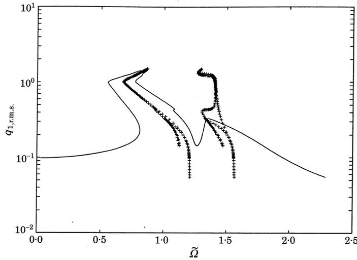
Figure 14. The frequency response of the system, showing the dependence of the natural frequencies on the response amplitude, given  $b_1 = 1.00$ ,  $b_2 = 0.10$ ,  $Q_{m,1} = Q_{m,2} = 0.50$ ,  $Q_{a,1} = 0.25$ ,  $Q_{a,2} = 0.00$  and  $\Delta\omega^* = 0.36$ . —, Response characteristics; +, backbone curve.
