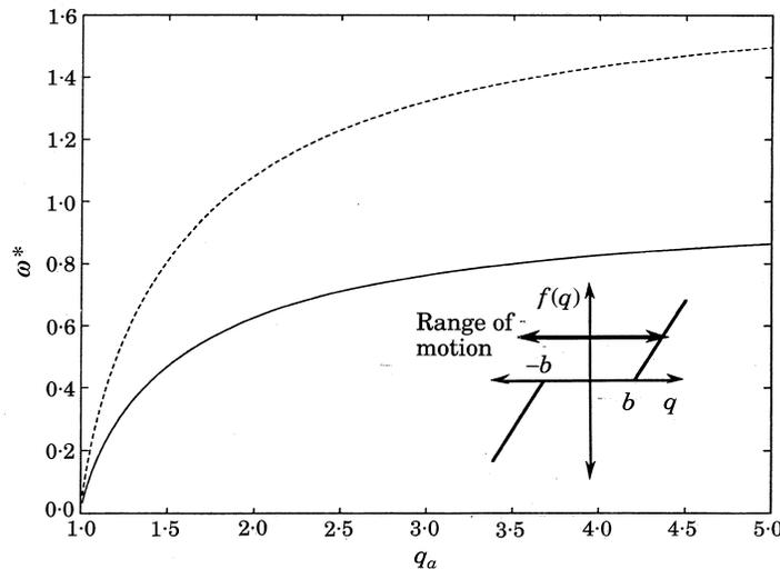
Figure 3. Variation of the natural frequencies of the system with response amplitude for a light mean load. —,  $\omega_1^*$ ; ----,  $\omega_2^*$ .
