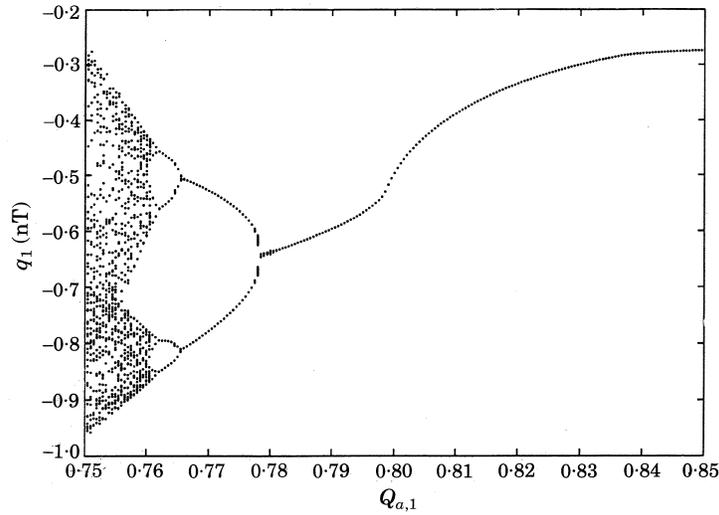
Figure 7. A bifurcation diagram of the system, given  $b_1 = b_2 = 1.00$ ,  $Q_{m,1} = Q_{m,2} = 0.50$ ,  $Q_{a,2} = 0.00$ ,  $\tilde{\Omega} = 0.20$  and  $\Delta\omega^* = 0.73$ .
