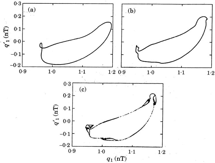
Figure 5. Poincaré maps for the system with  $b_1 = b_2 = 1.00$ ,  $Q_{m,1} = Q_{m,2} = 0.50$ ,  $Q_{a,2} = 0.00$ ,  $\tilde{Q} = 1.20$  and  $\Delta\omega^* = 0.73$ . (a)  $Q_{a,1} = 0.2125$ ; (b)  $Q_{a,1} = 0.2250$ ; (c)  $Q_{a,1} = 0.2313$ .
