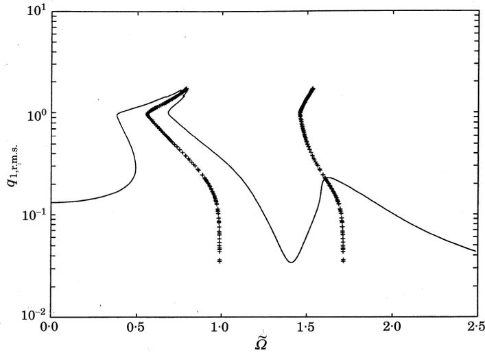
Figure 10. The frequency response of the system, showing the dependence of the natural frequencies on the response amplitude, given  $b_1 = 1.00$ ,  $b_2 = 0.00$ ,  $Q_{m,1} = Q_{m,2} = 0.50$ ,  $Q_{a,1} = 0.25$ ,  $Q_{a,2} = 0.00$  and  $\Delta\omega^* = 0.73$ . —, Response characteristics; +, backbone curve.
