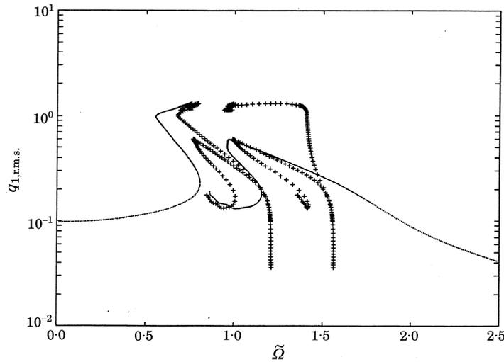
Figure 15. The frequency response of the system, showing the dependence of the natural frequencies on the response amplitude, given  $b_1 = 1.00$ ,  $b_2 = 0.50$ ,  $Q_{m,1} = Q_{m,2} = 0.50$ ,  $Q_{a,1} = 0.25$ ,  $Q_{a,2} = 0.00$  and  $\Delta\omega^* = 0.36$ . —, Response characteristics; +, backbone curve.
