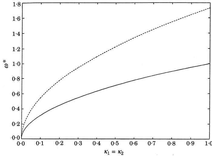
Figure 2. Variation of the natural frequencies of the linearized example with effective stiffness. —,  $\omega_1^*$ ; ---,  $\omega_2^*$ .
