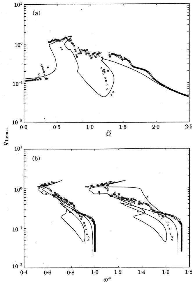
Figure 16. A comparison between the Galerkin method and classical numerical integration for the system, given  $Q_{m,1} = Q_{m,2} = 0.50$ ,  $Q_{a,1} = 0.25$ ,  $Q_{a,2} = 0.00$ ,  $b_1 = 1.00$  and  $b_2 = 0.50$ . (a) Response characteristics; (b) backbone curve. —, Galerkin method;  $\circ$ , classical numerical integration.
