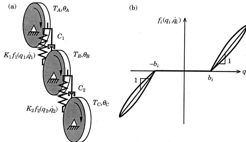
Figure 1. An example case: (a) A schematic of the reverse-idler gear pair, (b) backlash non-linearity with impact damping.
