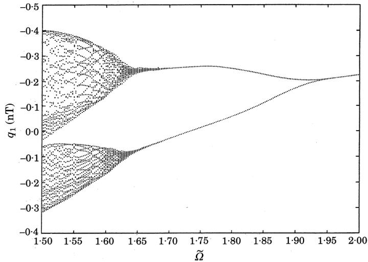
Figure 8. A bifurcation diagram of the system, given  $b_1 = 0.10$ ,  $b_2 = 1.00$ ,  $Q_{m,1} = Q_{m,2} = 0.50$ ,  $Q_{a,1} = 0.25$ ,  $Q_{a,2} = 0.00$  and  $\Delta\omega^* = 0.73$ .
