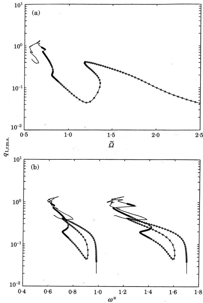
Figure 17. A comparison between the Galerkin method and the shooting method for the system, given  $Q_{m,1} = Q_{m,2} = 0.50$ ,  $Q_{a,1} = 0.25$ ,  $Q_{a,2} = 0.00$ ,  $b_1 = 1.00$  and  $b_2 = 0.50$ . (a) Response characteristics; (b) backbone curve. —, Galerkin method;  $\circ$ , shooting method.
