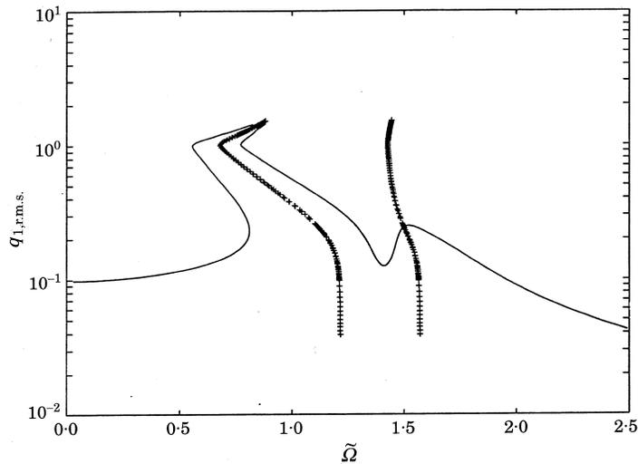
Figure 13. The frequency response of the system, showing the dependence of the natural frequencies on the response amplitude, given  $b_1 = 1.00$ ,  $b_2 = 0.00$ ,  $Q_{m,1} = Q_{m,2} = 0.50$ ,  $Q_{a,1} = 0.25$ ,  $Q_{a,2} = 0.00$  and  $\Delta\omega^* = 0.36$ . —, Response characteristics; +, backbone curve.
