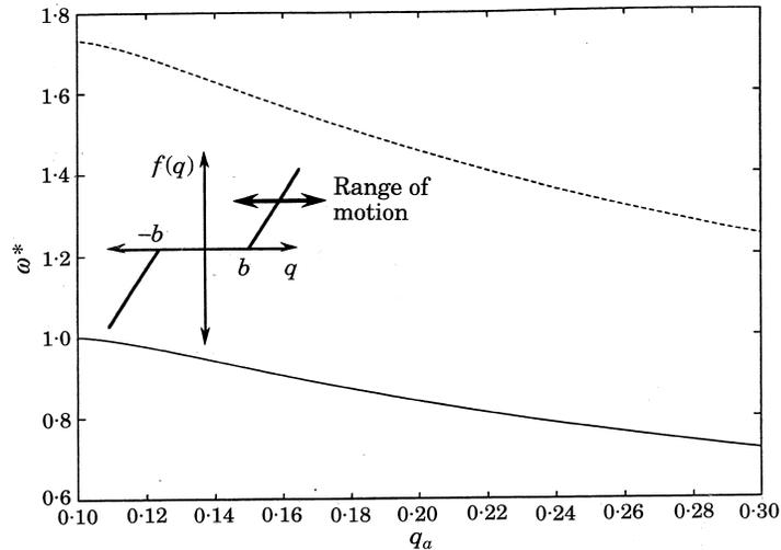
Figure 4. Variation of the natural frequencies of the system with response amplitude for a heavy mean load. —,  $\omega_1^*$ ; ----,  $\omega_2^*$ .
