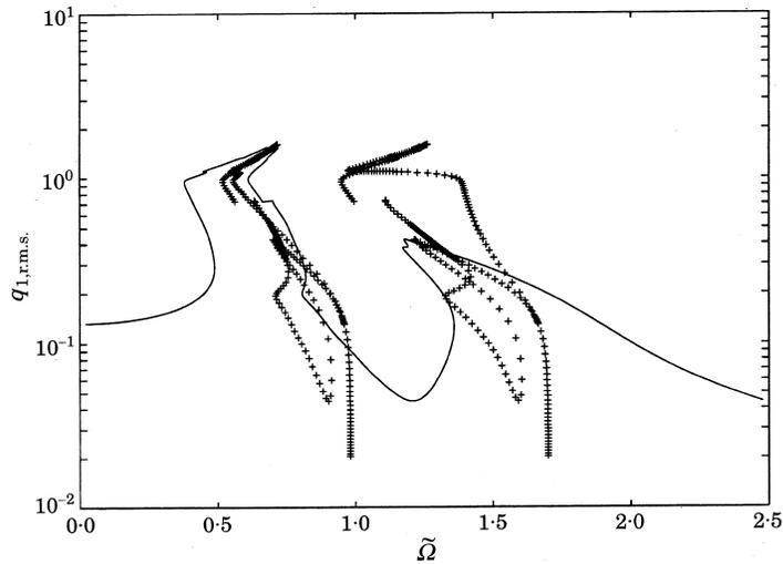
Figure 12. The frequency response of the system, showing the dependence of the natural frequencies on the response amplitude, given  $b_1 = 1.00$ ,  $b_2 = 0.50$ ,  $Q_{m,1} = Q_{m,2} = 0.50$ ,  $Q_{a,1} = 0.25$ ,  $Q_{a,2} = 0.00$  and  $\Delta\omega^* = 0.73$ . —, Response characteristics; +, backbone curve.
