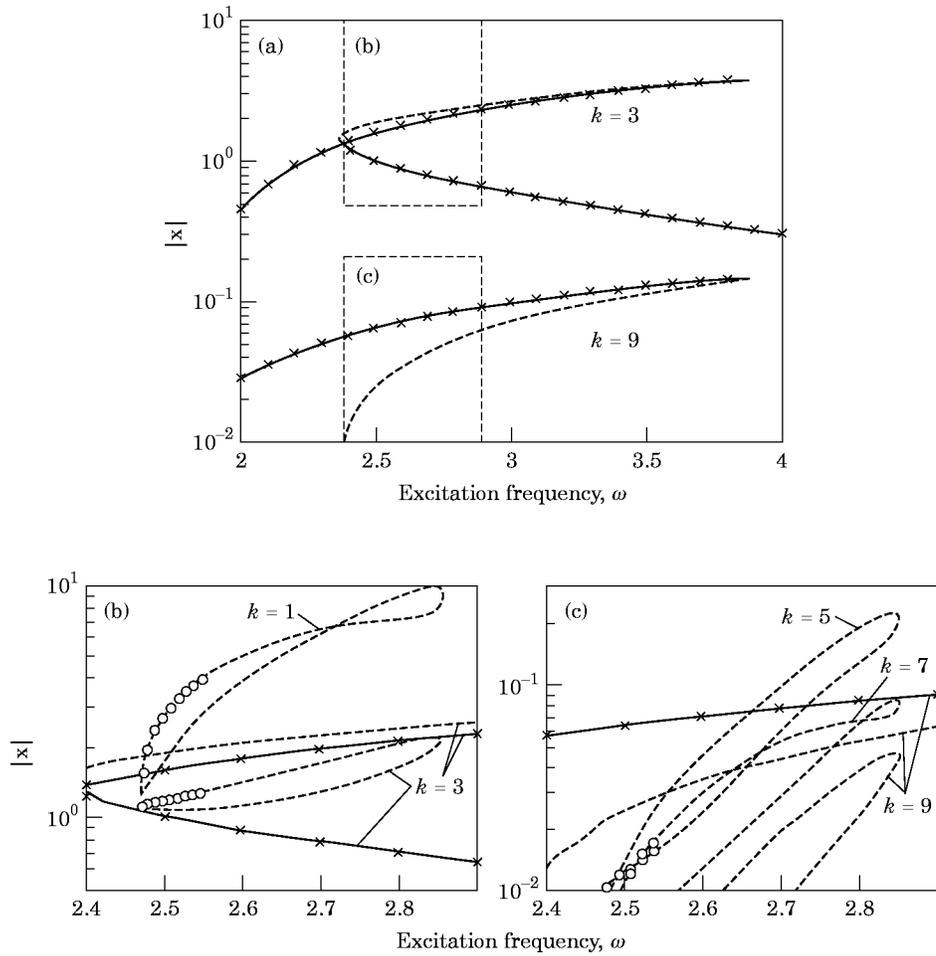
Figure 5. System response for digital computer study of example Case I. Selected super and subharmonic response of rigid mass motion  $x$ . Here  $m = 3$  and  $n = 15$ . Hence, the curve denoted by  $k$  is the  $k/3$ rd harmonic. Key: —, enhanced Galerkin method (--- unstable); x x x o o o, direct time integration. (a): Main solution path. (b) Close-up showing main and (c) secondary closed-loop solution paths.
