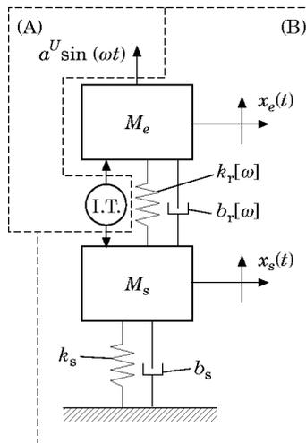
Figure 9. Example Case II: hydraulic engine mounting system. Here, I. T. refers to the inertia track, and subscripts  $e$ ,  $r$  and  $s$  refer to parameters associated with the engine, rubber part of the engine mount and the automotive chassis, respectively.
