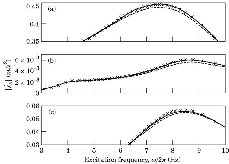
Figure 12. Hydraulic engine mounting system response with different mount rubber models. Solutions calculated with the enhanced Galerkin method. Here  $m = 1$  and  $n = 15$ . Hence, the curve denoted by  $k$  is the  $k$ th harmonic. Key: —, exact non-linear model; x x x, quasi-linear model; — — —, spectrally-invariant model. (a)  $k = 1$ , (b)  $k = 2$ , (c)  $k = 3$ .
