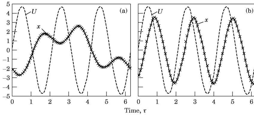
Figure 6. Time response of example Case I at  $\omega = 2.48$ . Key: —, direct time integration of  $x$ ; XXX, enhanced Galerkin Method of  $x$ ; ---, excitation force  $a^U \sin(\tau)$ . (a) Closed loop path stable solution. (b) Main path, large amplitude stable solution.
