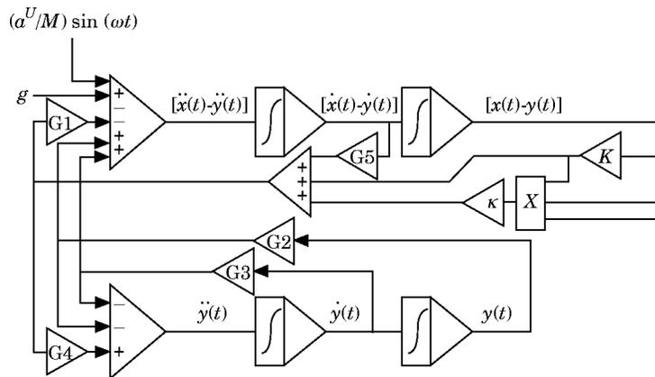
Figure 7. Diagram for analog computer simulation of Case I. See Table I for parameter values. Here  $G1 = (1/M) + (1/m_b)$ ,  $G2 = \omega_1^2$ ,  $G3 = 2\zeta_1\omega_1$ ,  $G4 = 1/m_b$ , and  $G5 = 2\zeta\sqrt{MK}$ .
