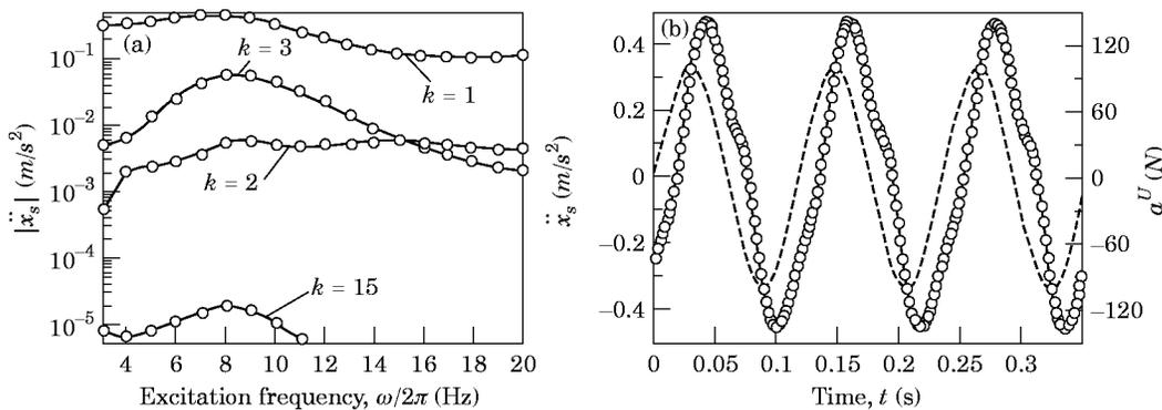
Figure 11. Hydraulic engine mounting system response with quasi-linear mount rubber model. (a) Selected superharmonic responses of chassis acceleration  $\ddot{x}_s$ . Hence  $m = 1$  and  $n = 15$ . Hence, the curve denoted by  $k$  is the  $k$ th harmonic. Key: —, enhanced Galerkin method; o o o, direct time integration. (b) Time response at  $\omega/2\pi = 8.5$  Hz of  $\ddot{x}_s$ . Key: —, direct time integration; o o o, enhanced Galerkin method; — — —, excitation force,  $a^U$ .
