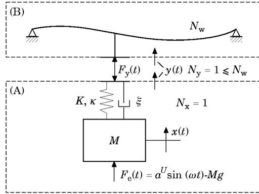
Figure 4. Example Case I: rigid body connected to a simply supported beam through a non-linear spring.
