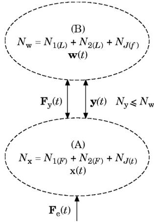
Figure 2. Subsystem structuring approach. Here,  $N_y$  denotes the dimension of the force/displacement connection between Sections (A) and (B).
