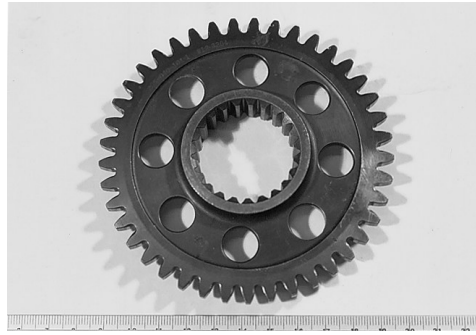
Figure 16. Gear from a helicopter tail rotor gearbox: case 14.
