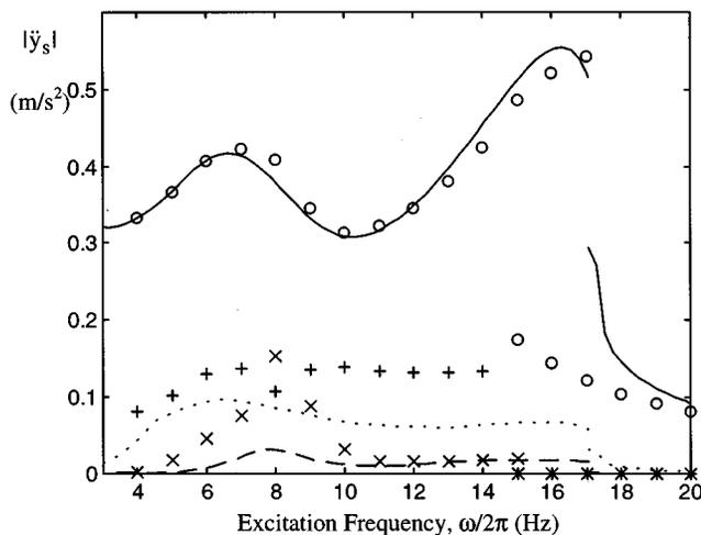
FIG. 5. Mounting system frequency response. Base acceleration at the excitation frequency and its first two harmonics,  $\ddot{y}_s$ , for  $\Delta_d=0.7$  mm and  $F_u(t)=100 \sin(\omega t)N$ . Key: Kinematic decoupler model,  $\circ$  1st,  $\times$  2nd,  $+$  3rd harmonics (numerical integration), polynomial-stiffness decoupler model with  $\gamma=3$ , — 1st, - - 2nd, . . . 3rd harmonics (Galerkin solution and numerical integration).
