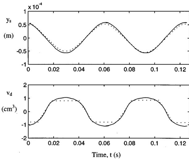
FIG. 4. Mounting system time response. Base motion,  $y_s(t)$ , and the total volume flow through the decoupler orifice,  $v_d(t)$ , for  $\Delta_d=0.7$  mm and  $F_u(t)=100 \sin(15.86 \times 2\pi t)N$  (large amplitude solution). Key: - - - kinematic decoupler model (numerical integration), — polynomial-stiffness decoupler model with  $\gamma=3$  (Galerkin solution and numerical integration).
