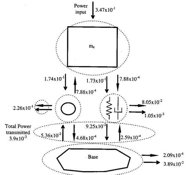
FIG. 7. Mounting system schematic showing directions of positive vibratory power flow for the SDOF base model and the polynomial-stiffness decoupler model with  $\gamma=3$ . Key:  $\rightarrow$  primary harmonic,  $\rightarrow\rightarrow$  higher harmonics.
