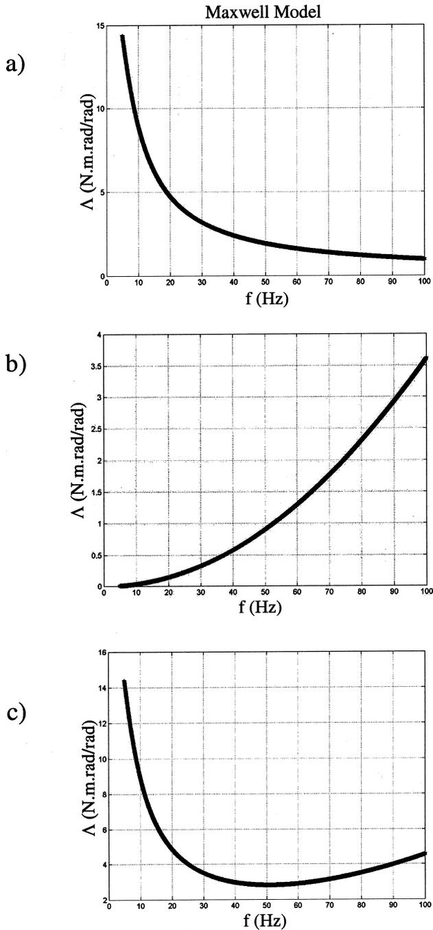
Fig. 11. Energy dissipation contribution from (a) visco-elastic model B only, (b) frequency-dependent dry-friction only, and (c) a combination of visco-elastic and frequency dependent dry-friction elements.
