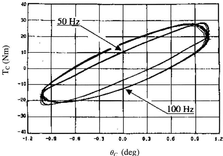
Fig. 4. Measured torque vs. displacement curve at excitation frequencies 50 and 100 Hz (with 2deg. peak-to-peak amplitude and 3deg. mean).
