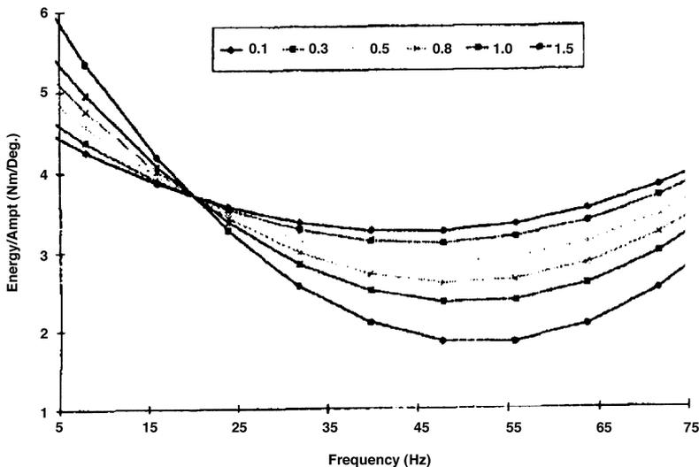
Fig. 5. Measured energy dissipation per unit amplitude ( $\Delta$ ) of clutch damper vs. frequency ( $f$ ), as extracted from [10]. Here the excitation amplitudes ( $\theta_c$ ) vary from 0.1 to 1.5 degrees.
