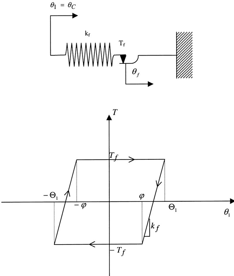
Fig. 6. Torque vs. excitation displacement  $\theta_1$  for the dry friction element.
