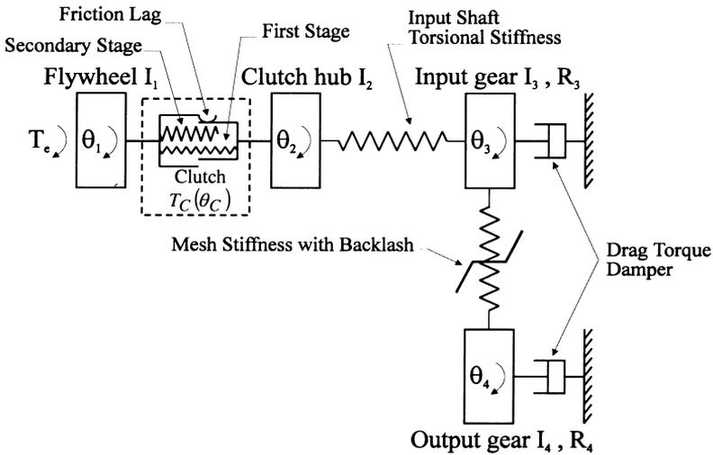
Fig. 1. Vehicle gearbox model used for gear rattle analysis.
