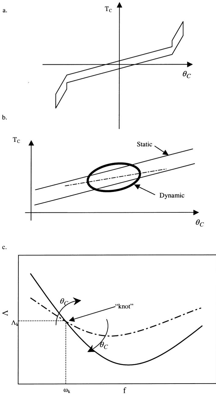
Fig. 2. Typical clutch properties. (a) Static torque vs. displacement. (b) Dynamic torque vs. displacement. (c) Energy dissipation per unit amplitude for various displacement amplitudes  $\theta_C$ . Here,  $f$  is the frequency in Hz.
