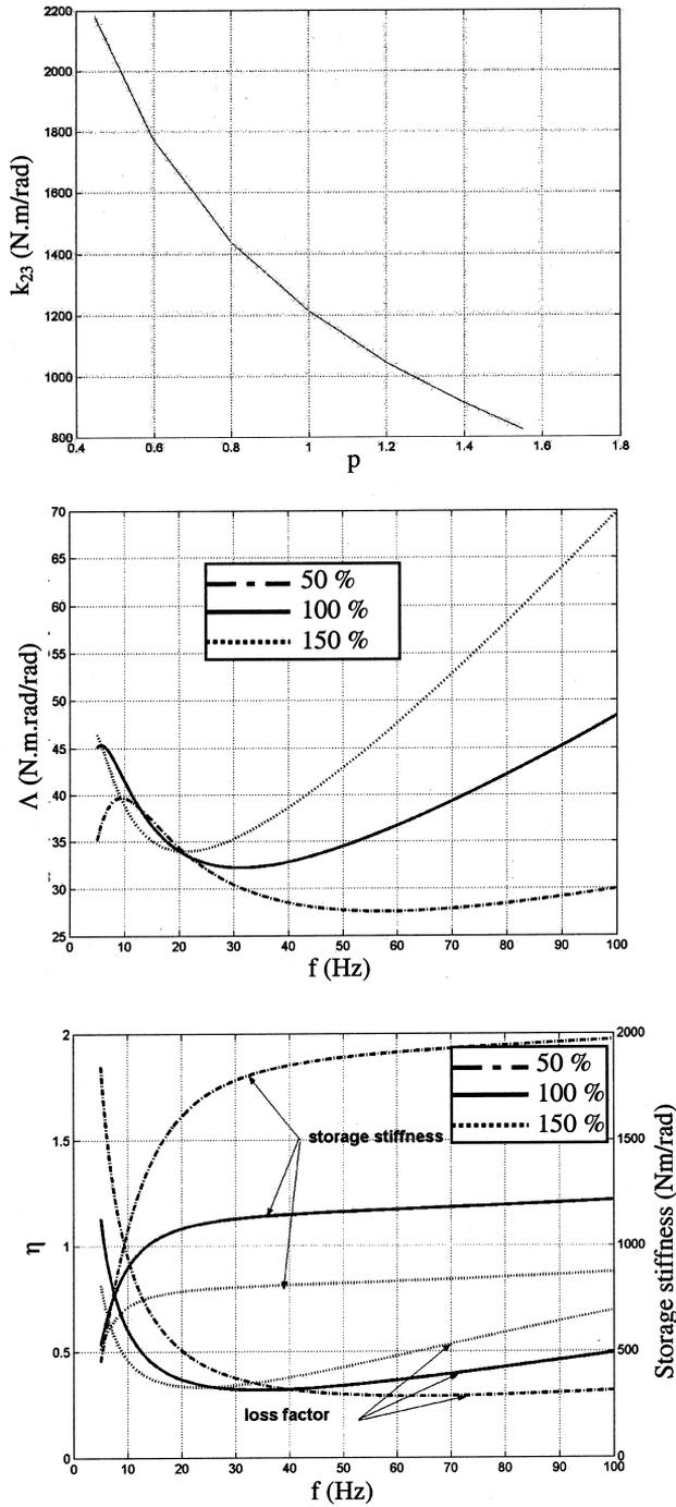
Fig. 12. Study of amplitude dependence for parameter  $k_{23}$  of model D.
