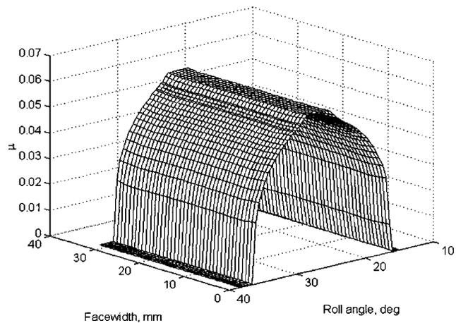
Fig. 2 Typical variation in  $\mu$  over the entire surface of a spur gear tooth
