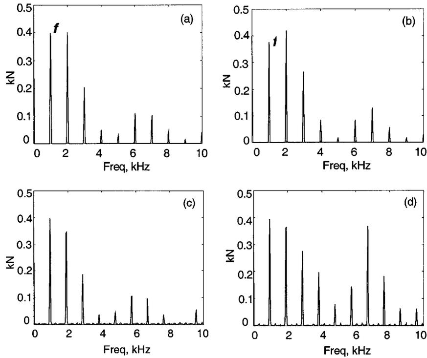
**Fig. 5 Spectra of total friction force on when static and dynamic mesh forces are considered at  $\Gamma=1.532$ ,  $\mu=0.1$  and  $\zeta=0.01$ . (a)  $F_f$  calculated using  $N$ , at  $\Omega_p=2400$  rpm (nonresonant condition); (b)  $F_f$  using  $F_{mesh}$ , at  $\Omega_p=2400$  rpm; (c)  $F_f$  using  $N$ , at  $\Omega_p=2300$  rpm (resonant condition); (d)  $F_f$  using  $F_{mesh}$ , at  $\Omega_p=2300$  rpm.**
