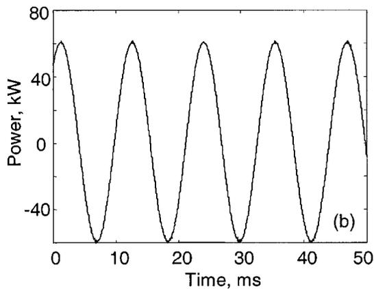
**Fig. 7** Input power to the geared system. (a) With constant output and input torques, mean power=0; (b) With constant input torque and spring attached to output gear, mean power =629 Watts (equivalent to energy loss due to friction).
