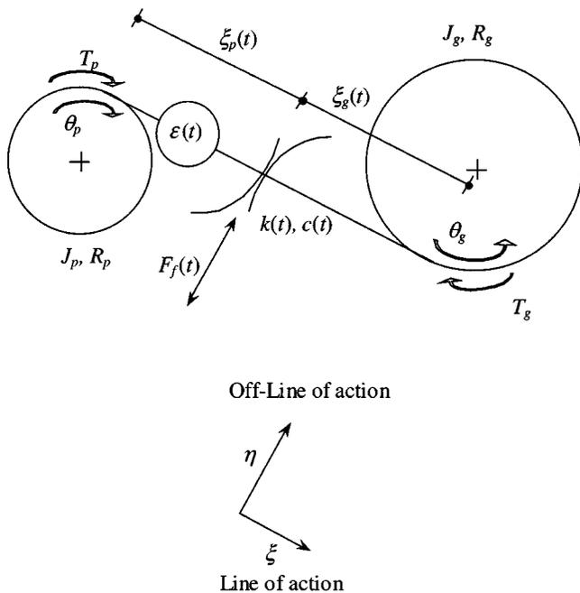
Fig. 1 Torsional model of gear pair with friction force
