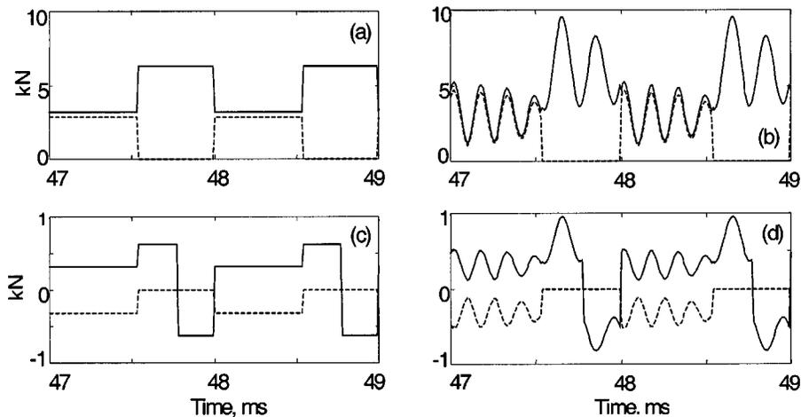
**Fig. 4 Simulated mesh and friction forces on the two teeth when static and dynamic mesh forces are considered at  $\Gamma=1.532$ ,  $\mu=0.1$ ,  $\zeta=0.01$ ,  $\Omega_p=2400$  rpm (non-resonant condition). (a) Mesh load using  $N$ ; (b) Mesh load using  $F_{\text{mesh}}$ ; (c)  $F_f$  using  $N$ ; (d)  $F_f$  using  $F_{\text{mesh}}$ . Key: - - - 1st tooth in mesh, — 2nd tooth in mesh (2 mesh cycles shown).**
