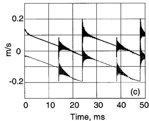
**Fig. 8** Variation of sliding speed for the three friction models. (a)  $V_s$  for quasistatic case; (b)  $V_s$  for LTV model; (c)  $V_s$  with nonlinear friction. Key: — 1st tooth, - - - 2nd tooth.
