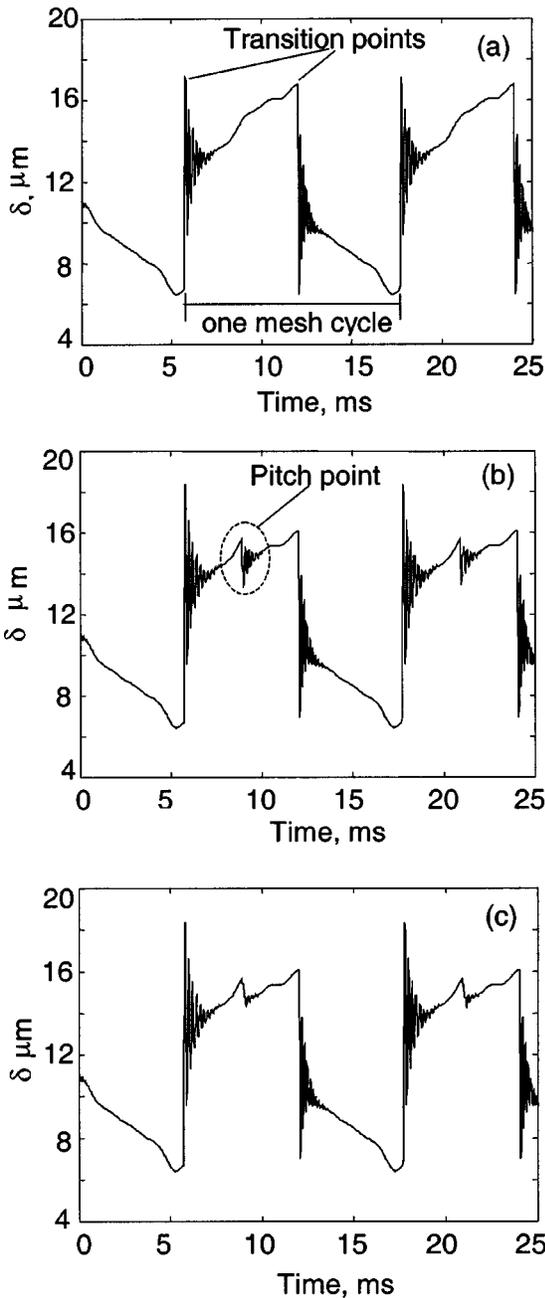
Fig. 11 Dynamic response for the three friction models in terms of  $\delta$ , at  $\Omega_p=200$  rpm,  $\zeta=0.05$ . (a) LTV system with  $\mu_0=0$ ; (b) LTV system with  $\mu_0=0.1$ ; (c) NLTV system with  $\mu_0=0.1$ .
