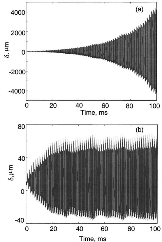
Fig. 12 Dynamic response  $\delta(t)$  with LTV analysis, near resonance conditions for  $\zeta=0.001$ ,  $\mu=0.1$ ,  $\Omega_p=1490$  rpm,  $\Gamma=1.473$ . (a) LTV system; (b) NLTV system.
