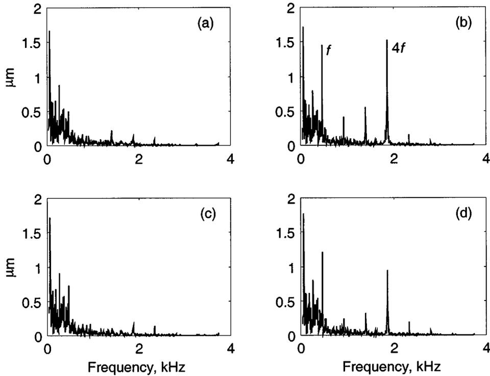
**Fig. 3 Measured pinion deflection in traction ( $\xi$ ) and sliding ( $\eta$ ) direction for  $T_p=102$  Nm,  $\Omega_p=1000$  rpm. (a) Low  $\eta_0$  lubricant,  $\xi$ -direction; (b) Low  $\eta_0$  lubricant,  $\eta$ -direction; (c) High  $\eta_0$  lubricant,  $\xi$ -direction; (d) High  $\eta_0$  lubricant,  $\eta$ -direction.**
