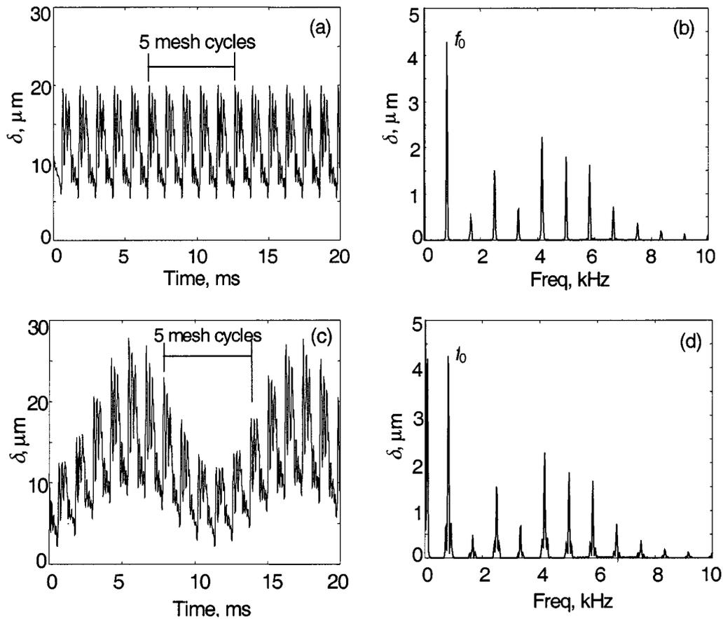
**Fig. 6 Dynamic response  $\delta(t)$  for 2000 rpm,  $\zeta=.05$ ,  $\Gamma=1.473$ ,  $\mu=0.1$ ,  $k/k_b=5 \times 10^5$  (a) Semi-positive definite system: time response; (b) Semi-positive definite system: frequency spectrum; (c) Positive definite system with extra spring: time response; (d) Positive definite system with extra spring: frequency spectrum.**
