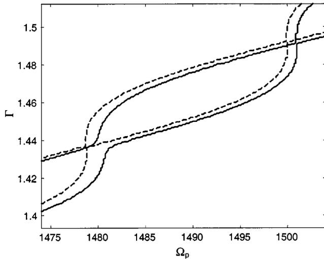
Fig. 13 Effect of Coulomb friction on instability zone, (—) with friction, (---) without friction (area enclosed within the curves is the unstable zone)
