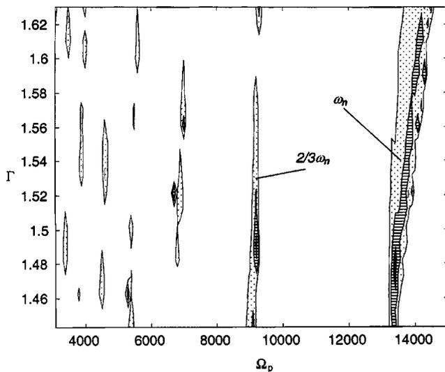
Fig. 14 Contours plots for the ratio  $\gamma$  of magnitude of  $\delta$  between LTV and NLTV models, key:  $\dots$   $\gamma=3$ ,  $\text{---}$   $\gamma=100$ ,  $\blacksquare$   $\gamma=100,000$ .
