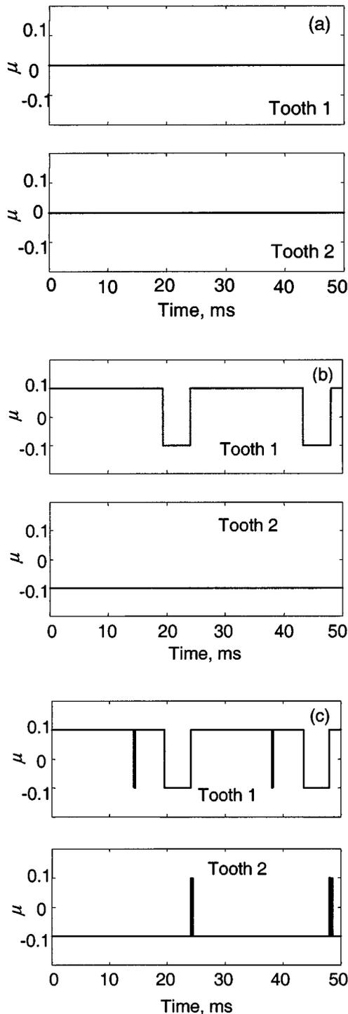
**Fig. 9** Variation in coefficient of friction for different models at  $\Omega_p=100$  rpm,  $\mu=0.1$ ,  $\Gamma=1.590$ ,  $\zeta=0.01$ . (a) No friction; (b) Assumed variation corresponding to Fig. 7(b); (c) Actual variation corresponding to Fig. 7c.
