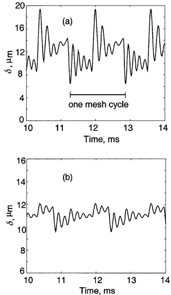
**Fig. 10** Sample response for  $\delta$  due to individual and combined excitations. (a) All excitations combined; (b) Only friction excitation  $T_f(t)$ .
