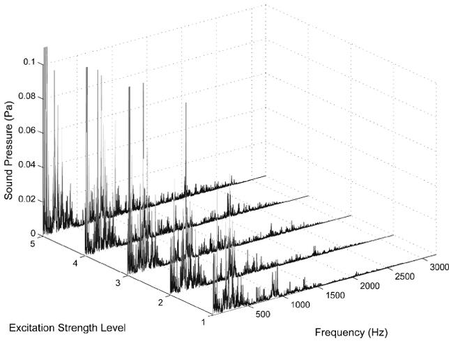
Fig. 5—Sound pressure spectra (on narrow band basis), measured in the receiver room at P1, for 5 excitation levels. Source strength level settings are given by the following combination of voltages (V). Level 1: Pump 2 V, Motor 40 V; Level 2: Pump 4 V, Motor 45 V; Level 3: Pump 6 V, Motor 50 V; Level 4: Pump 8 V, Motor 55 V; Level 5: Pump 10 V, Motor 60 V.
