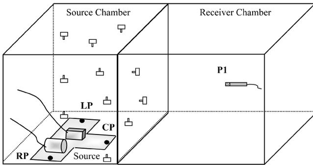
Fig. 1—Schematic of the experimental two-chamber system. Vibration from the source unit is transmitted to the receiver microphone location P1 as structure-borne noise through three hard paths (mounts); left, center and right paths are denoted as LP, CP and RP respectively. Many accelerometers are installed in walls of the source chamber.
