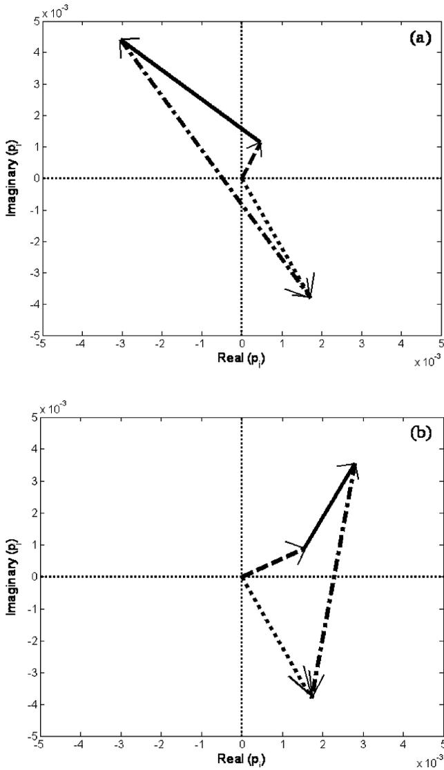
Fig. 11—Vectorial representations of the partial sound pressures at 163 Hz based on measured velocities: (a) with impedance method (8); (b) with mobility method (7). Key: - - - - -, total sound pressure, - - -, left path; —, center path; · · · · ·, right path.
