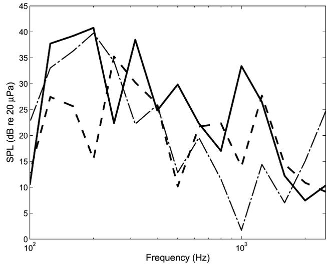
Fig. 12—Path rank orders based on partial sound pressures (on one third octave band basis) obtained via mobility method (7) with measured velocities. Key: - - -, left path; —, center path; · · · · ·, right path.
