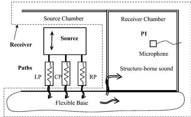
Fig. 3—Structure-borne noise transmission paths of the experimental system. Left, center and right paths are connected to the source chamber base plate via hard mounts. Receiver is denoted by the dotted line.
