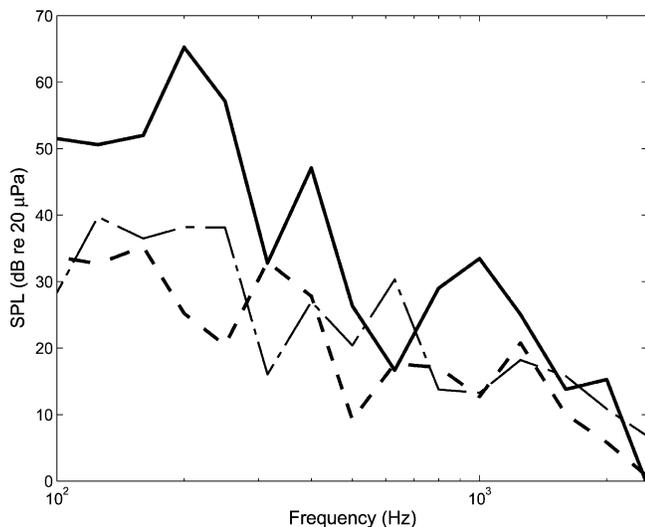
Fig. 9—Estimated partial sound pressures (on one third octave band basis) by using the mobility method with measured forces (5).
