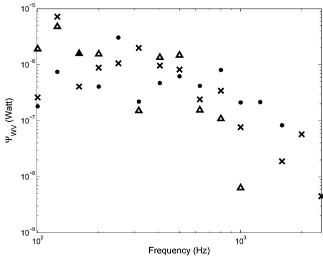
Fig. 15—Weighted mean-square velocity ( $\Psi_{WV}^2$ ) components (on one third octave band basis) for 3 paths. Key: •, left path; x, center path; Δ, right path. Negative values are not shown here.
