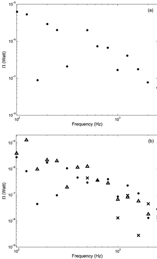
Fig. 13—Power flow through paths (on one third octave band basis): (a) total power flow; (b) power flow through each path. Key: (a) •, total power flow; (b) •, left path; x, center path; Δ, right path. Negative values are not shown here.
