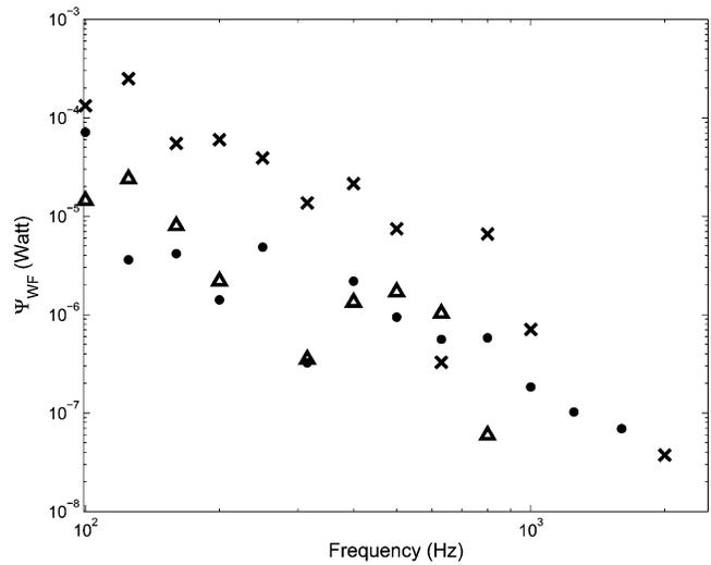
Fig. 14—Weighted mean-square path force ( $\Psi_{WF}^2$ ) components (on one third octave band basis) for 3 paths. Key: •, left path; x, center path; Δ, right path. Negative values are not shown here.
