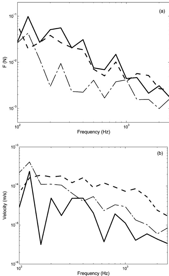
Fig. 8—Measured path force (a) and velocity (b) spectra (on one third octave band basis). Key: - - -, left path; —, center path; · - · - ·, right path.
