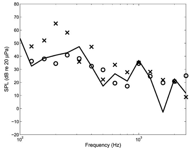
Fig. 7—Receiver room sound pressure levels (SPL) on one third octave band basis. Key: —, measured (direct) SPL; x, estimated SPL ( $p_{FY} = p_{FZ}$ ) using indirect method based on measured forces ((5) or (6)); o, estimated SPL ( $p_{VY} = p_{VZ}$ ) using indirect method I based on measured velocities ((7) or (8)).
