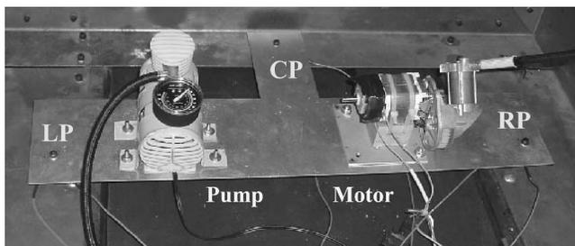
Fig. 2—Source unit consisting of an air pump, a motor and a T-shaped base plate. This unit is installed near the floor of the source chamber base plate using three mounts (or paths LP, CP and RP).
