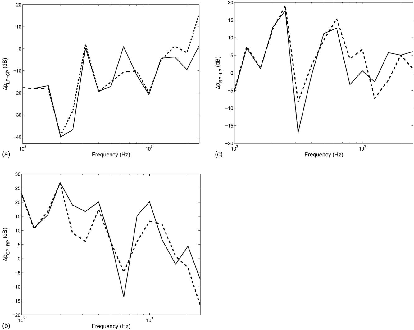
Fig. 10—Relative partial sound pressures (on one third octave band basis) obtained using mobility (5) or impedance (6) method with measured forces: (a)  $\Delta p_{LP-CP}$ ; (b)  $\Delta p_{CP-RP}$ ; (c)  $\Delta p_{RP-LP}$ . Key: —, mobility method; - - -, impedance method.
