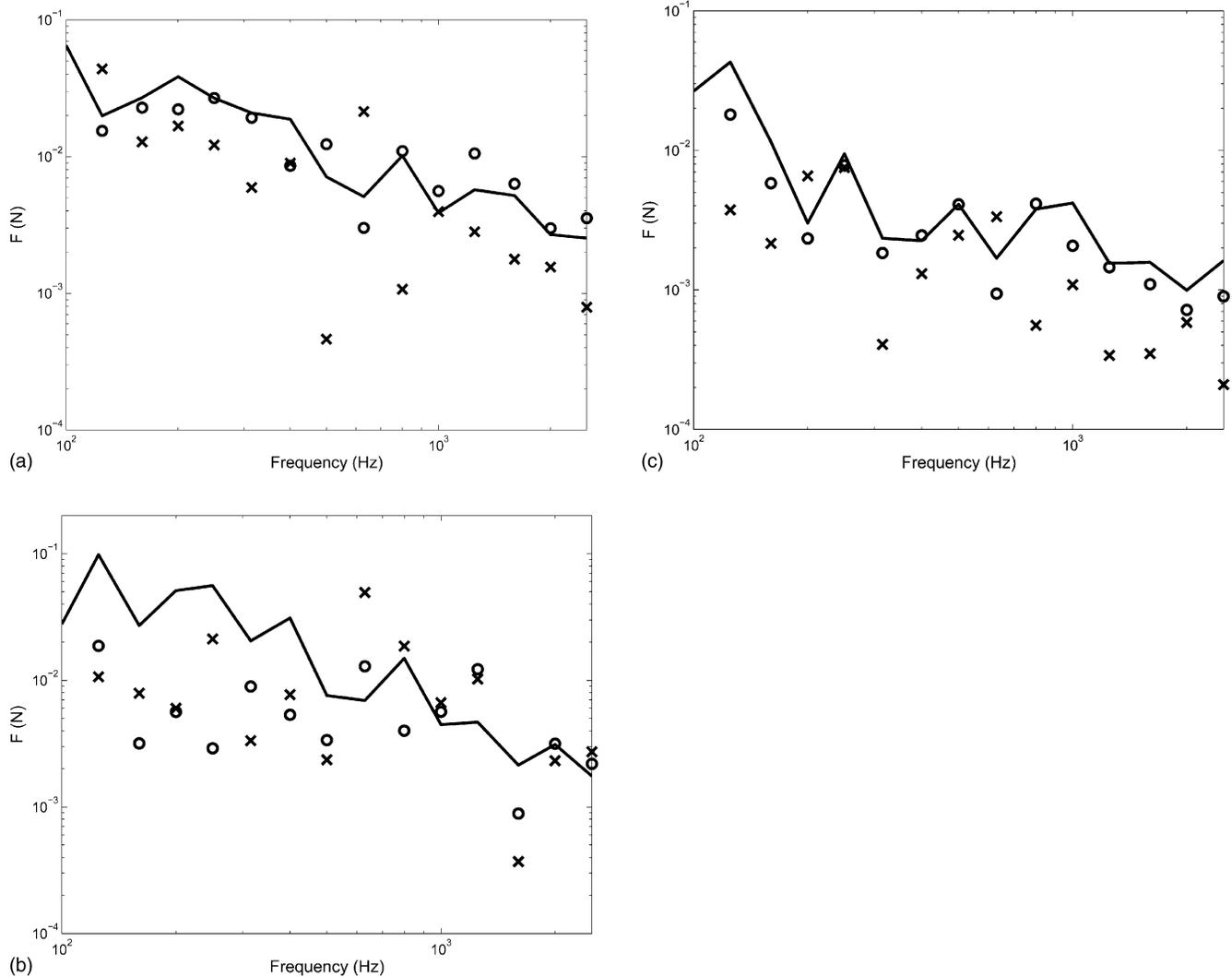
Fig. 6—Interfacial force spectra (on one third octave band basis) for 3 paths: (a) left path; (b) center path; (c) right path. Key: —, measured (direct) force; o, estimated force via the indirect method I; x, estimated force via the indirect method II.
