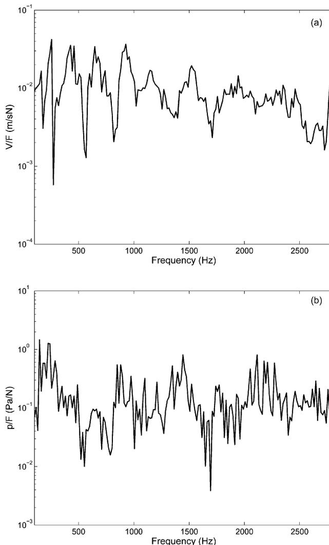
Fig. 4—Measured structural and acoustic frequency response functions (FRF) on a narrow band basis: (a) driving point mobility at the left path; (b) acoustic FRF ( $p/F$ ) with sound pressure in the receiver room (at P1) and force at the center path.
