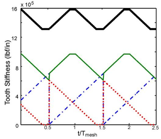
**Fig. 4 Predicted tooth stiffness functions. Key: blue dashed-dotted line, tooth pair 0; green solid line, tooth pair 1; red dotted line, tooth pair 2; thick solid line, combined tooth pair stiffness.**
