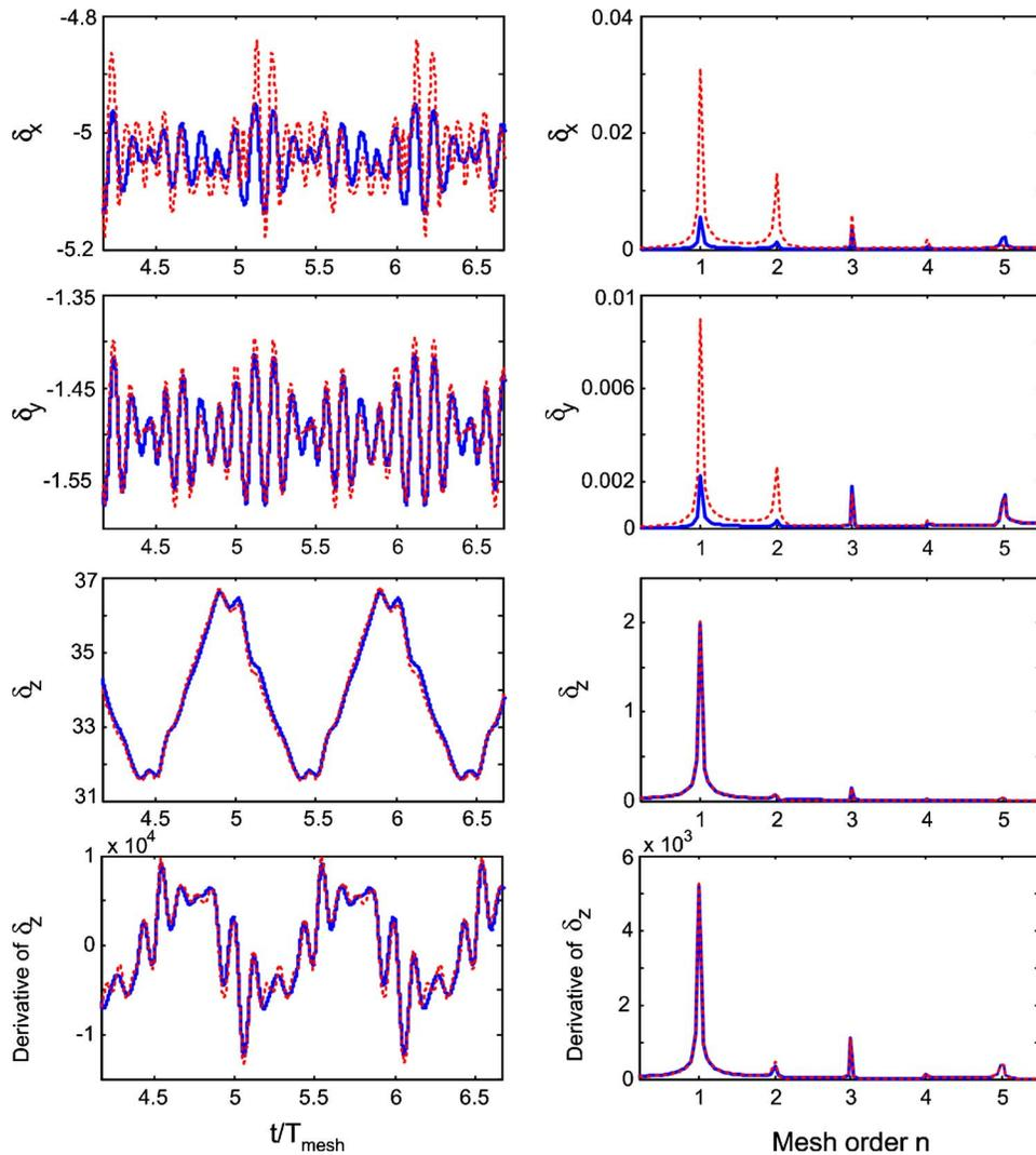
**Fig. 8 Time and frequency domain responses of composite displacements  $\delta_x$ ,  $\delta_y$ ,  $\delta_z$ , and velocity  $\dot{\delta}_z$  at  $T_p=2000$  lbf/in. and  $\Omega_p=1000$  rpm. All motions are normalized with respect to  $39.37 \mu\text{in.}$  ( $1 \mu\text{m}$ ) or  $39.37 \mu\text{in./s}$  ( $1 \mu\text{m/s}$ ). Key: blue solid line  $\mu=0.01$ , red dotted line  $\mu=0.1$ .**
