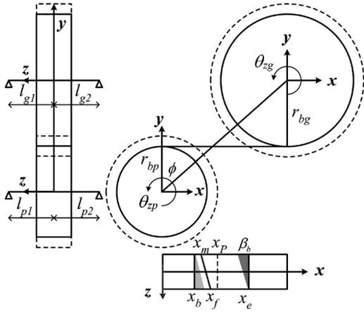
Fig. 1 Schematic of the helical gear pair system
