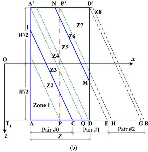
**Fig. 3 Contact zones at the beginning of a mesh cycle: (a) in the helical gear pair and (b) contact zones within contact plane. Key: PP' is the pitch line; AA' is the face width  $W$ ; AD is the length of contact zone  $Z$ .**
