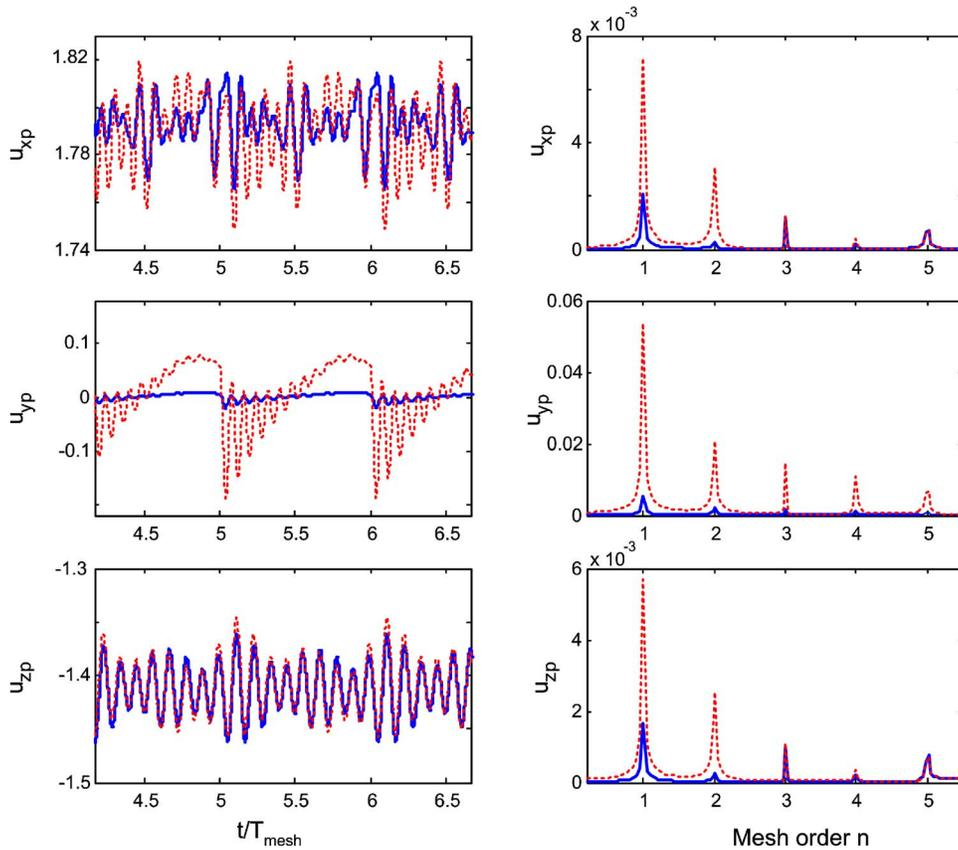
**Fig. 6 Time and frequency domain responses of translational pinion displacements  $u_{xp}$ ,  $u_{yp}$ ,  $u_{zp}$  at  $T_p=2000$  lb/in. and  $\Omega_p=1000$  rpm. All displacements are normalized with respect to  $39.37 \mu\text{in.}$  ( $1 \mu\text{m}$ ). Key: blue solid line  $\mu=0.01$ , red dotted line  $\mu=0.1$ .**
