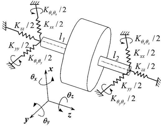
**Fig. 5 Schematic of the bearing-shaft model. Here, the shaft and bearing stiffness elements are assumed to be in series to each other. Only pure rotational or translational stiffness elements are shown. Coupling stiffness terms  $K_{x\theta_y}$ ,  $K_{x\theta_x}$  are not shown.**
