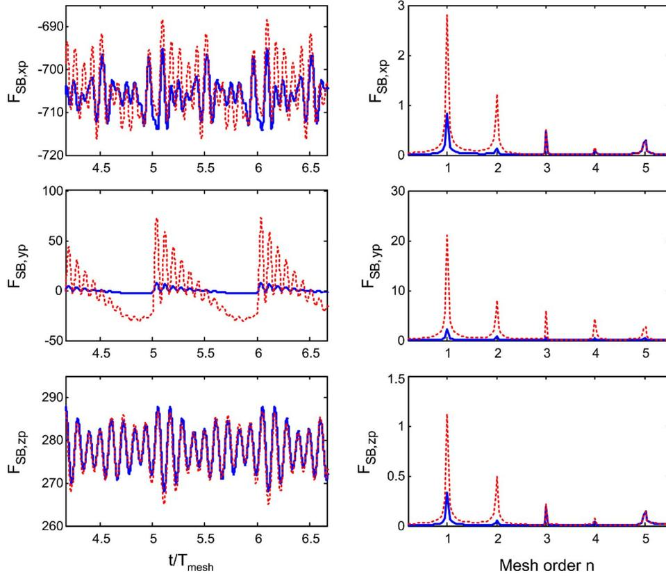
**Fig. 7 Time and frequency domain responses of pinion bearing forces  $F_{SB,xp}$ ,  $F_{SB,yp}$ , and  $F_{SB,zp}$  at  $T_p=2000$  lb/in and  $\Omega_p=1000$  rpm. All forces are normalized with respect to 1 lbf. Key: blue solid line  $\mu=0.01$ , red dotted line  $\mu=0.1$ .**
