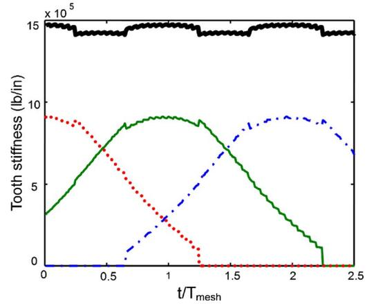
Fig. 2 Tooth stiffness function calculated using Eq. (1) based on the FE/CM code [11]. Key: red dotted line, tooth pair 0; green solid line, tooth pair 1; blue dashed-dotted line, tooth pair 2; thick solid line, combined tooth pair stiffness.
