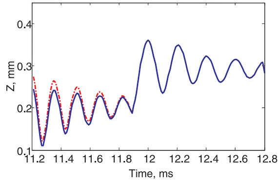
Figure 7. Calculated width of the instantaneous contact zone for the example of Table 1. Key: —, second pair of teeth; - - - - - , first pair of teeth.
