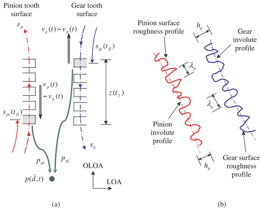
Figure 6. Simplified sound source as generated by the surface roughness. (a) Schematic of sound radiation due to asperity impacts within the gear contact zone; (b) surface roughness description.
