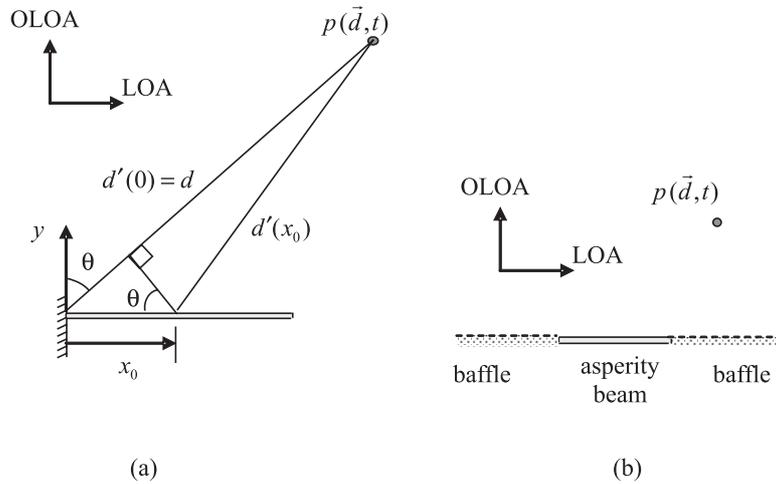
Figure 2. Sound radiation from an asperity modeled as a cantilever beam (clamped to the gear tooth surface). (a) Schematic for sound radiation calculation. (b) Baffle configuration.
