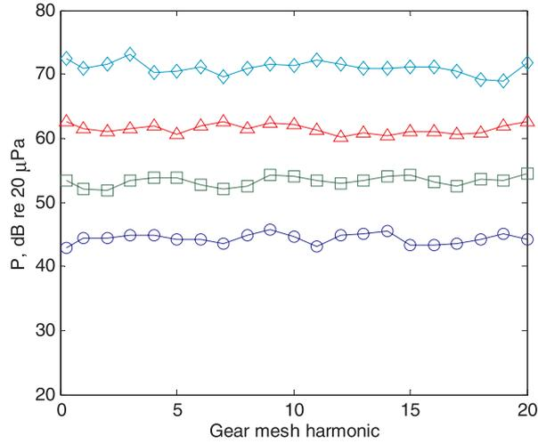
Figure 10. Effect of operating speed on sound pressure spectra given  $h = 1 \mu\text{m}$ . Key:  $\circ$ , 500 rpm;  $\square$ , 1000 rpm,  $\triangle$ , 2000 rpm,  $\diamond$ , 4000 rpm.
