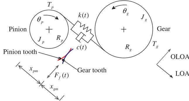
Figure 5. Gear dynamic model with time-varying mesh parameters and sliding friction.
