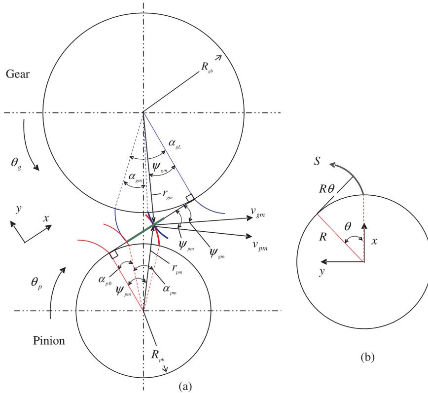
Figure 3. Gear kinematic model. (a) Key roll angles; (b) gear involute coordinate and parameters.
