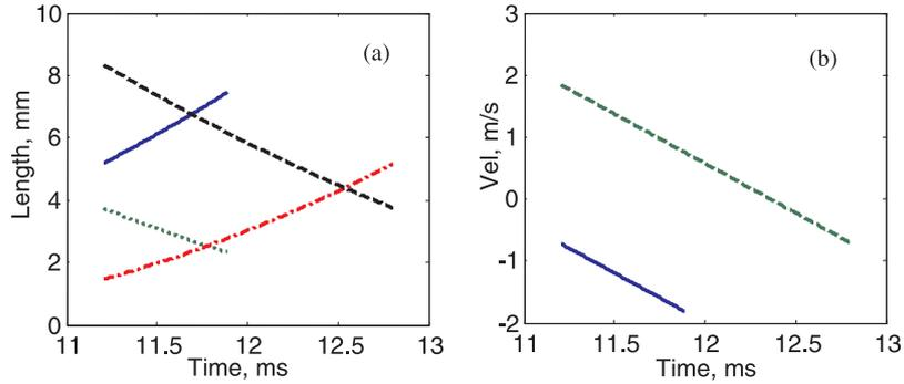
Figure 4. Gear tooth involute parameters for one mesh period given constant operating speeds. (a) Mesh location at involute coordinates. Key: —, 1st tooth of pinion; ·····, 1st tooth of gear; - - - - , 2nd tooth of pinion; - - - - , 2nd tooth of gear. (b) Sliding speed of meshing teeth in OLOA direction. Key: —, 1st teeth pair; ·····, 2nd teeth pair.
