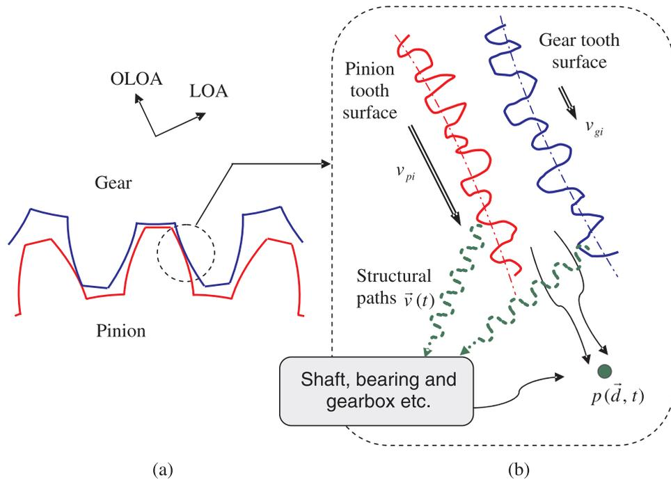
Figure 1. Problem formulation. (a) Spur gear pair in mesh with given surface roughness; (b) related air-borne and structure-borne noise generation. Here, velocity magnitudes ( $v_{pi}$  and  $v_{gi}$ ) of gear tooth surfaces in the sliding direction are depicted by the length of arrows. Further, the undulated surface-induced vibration transmitted to the surrounding structures is denoted by  $\vec{v}(t)$ . Key: LOA = line of action; OLOA = off-line of action.
