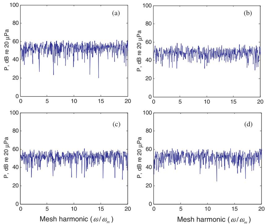
Figure 9. Sound pressure spectra at 1500 rpm given  $h = 1 \mu\text{m}$ . (a) Sound pressure from pinion of the first tooth pair; (b) gear of the first tooth pair; (c) pinion of the second tooth pair; (d) gear of the second tooth pair.
