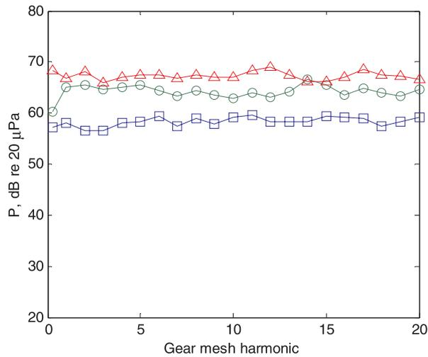
Figure 11. Effect of surface roughness height ( $h$ ) on sound pressure spectra at 1500 rpm. Key:  $\square$ ,  $h = 1 \mu\text{m}$ ;  $\circ$ ,  $h = 2.5 \mu\text{m}$ ,  $\triangle$ ,  $h = 5 \mu\text{m}$ .
