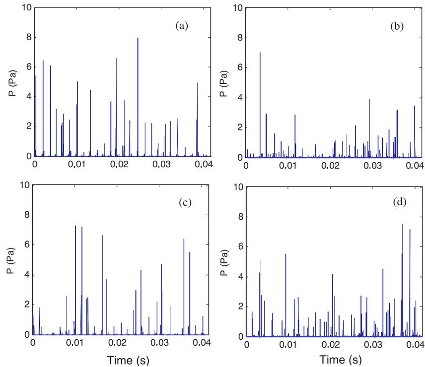
Figure 8. Time histories of the radiated sound pressures at 1500 rpm given surface roughness height of  $h = 1 \mu\text{m}$ . (a) Sound pressure from pinion of the first tooth pair; (b) gear of the first tooth pair; (c) pinion of the second tooth pair; (d) gear of the second tooth pair.
