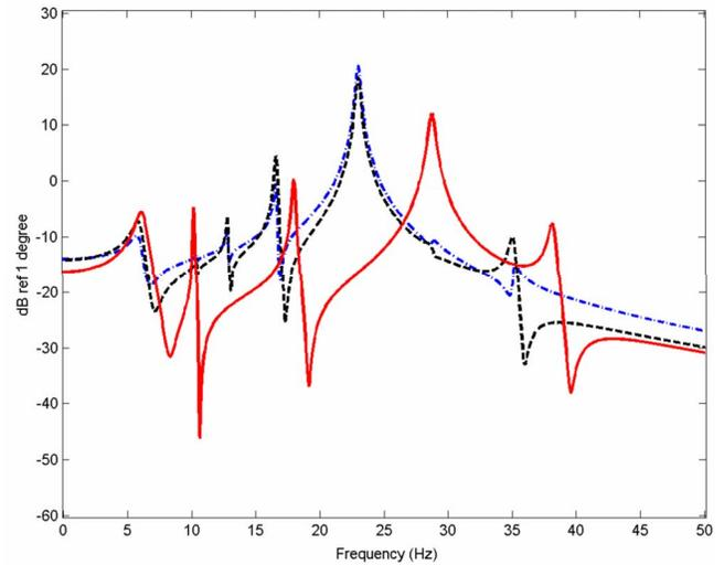
Fig. 10—Effect of orientation angle on frequency responses in roll direction ( $\theta_X(\omega)$ ) of the active powertrain system (Fig. 6) given harmonic torque excitation with 100Nm amplitude. One active mount of Fig. 4 is placed at location #1. Key: --- (blue),  $X_A=0$  mm,  $\phi=30^\circ$ ; --- (black),  $X_A=1.5$  mm with  $\phi_A=180^\circ$ ,  $\phi=30^\circ$ ; — (red),  $X_A=1.5$  mm with  $\phi_A=180^\circ$ ,  $\phi=0^\circ$  (vertical).
