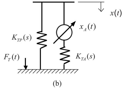
Fig. 2—Passive and active engine mounts given displacement input  $x(t)$ . (a) Passive mount; (b) Active mount with piston displacement type input ( $x_A(t)$ ). In both cases, force transmitted to the rigid base is  $F_T(t)$ . Stiffness terms are given in the Laplace domain.
