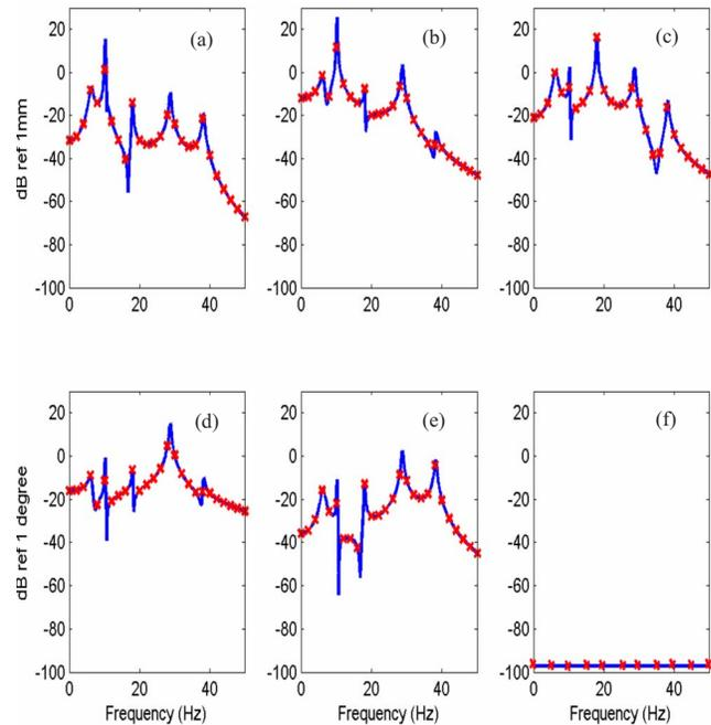
Fig. 8—Frequency response of an active powertrain mounting system of Fig. 6 given harmonic torque with 100 N m amplitude. One active mount of Fig. 4 is placed at location #1 and the rest are passive mounts. (a)  $X(\omega)$ ; (b)  $Y(\omega)$ ; (c)  $Z(\omega)$ ; (d)  $\theta_x(\omega)$ ; (e)  $\theta_y(\omega)$ ; (f)  $\theta_z(\omega)$ . Key: — (black), analytical (modal expansion method);  $\times$  (red), numerical (direct inversion method).
