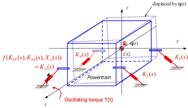
Fig. 1—Multi-degree-of-freedom powertrain isolation system with one active mount and three passive mounts. Each mount is described by tri-axial elements with frequency dependent stiffness  $k(\omega)$  and damping  $c(\omega)$  properties. Here,  $K_i(s)$  ( $i = 2, 3, \text{ and } 4$  (here  $n$  is the number of mounts)) and  $K_A(s)$  are the dynamic stiffness terms of passive and active elements (in a specific direction) respectively.
