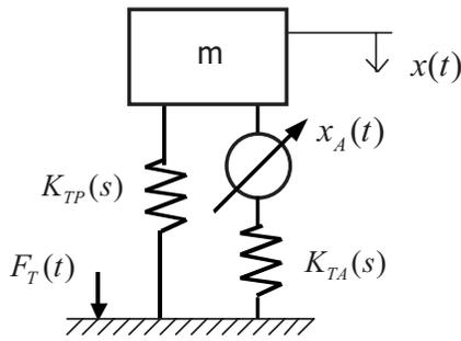
Fig. 3—Single-degree-of-freedom system with an active mount.
