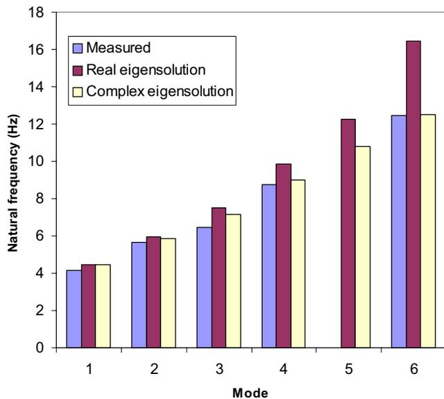
Fig. 7—Comparison of calculated (using both real and complex eigensolution methods) and measured<sup>11</sup> natural frequencies for a V6 diesel engine.
