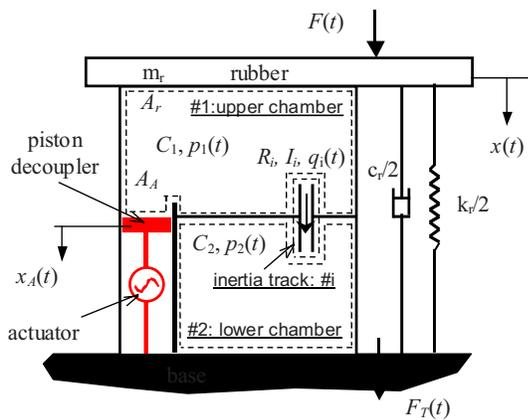
Fig. 4—Schematic of an active engine mount based on hydraulic mount. Here,  $C_1$  and  $C_2$  are the compliances of upper and lower chambers,  $p_1(t)$  and  $p_2(t)$  are the chamber pressures,  $R_i$ ,  $I_i$ , and  $q_i(t)$  are the fluid resistance, inertance, and flow rate in the inertia track,  $A_r$  is the equivalent piston area of rubber,  $A_A$  is the actuator piston area, and  $k_r$  and  $c_r$  are the rubber stiffness and viscous damping terms (Voigt model assumed).
