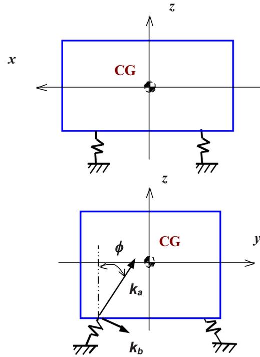
Fig. 6—Focalized powertrain mounting system (6-DOF). Here,  $k_a$  is the principal compressive stiffness and  $k_b$  is the principal shear stiffness.
