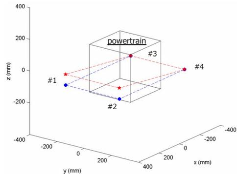
Fig. 11—Mount locations for coupled and decoupled powertrain of Fig. 6 given harmonic torque excitation. One active mount (with inactive actuator) of Fig. 4 is placed at location #1 and the rest are passive mounts; motions are decoupled by adjusting location and orientation angle of mount #1. Key: ★ (red), TRA decoupled ( $\phi=0^\circ$ ,  $r_z=0$  mm); ● (blue), Coupled ( $\phi=15^\circ$ ,  $r_z=-68$  mm)
