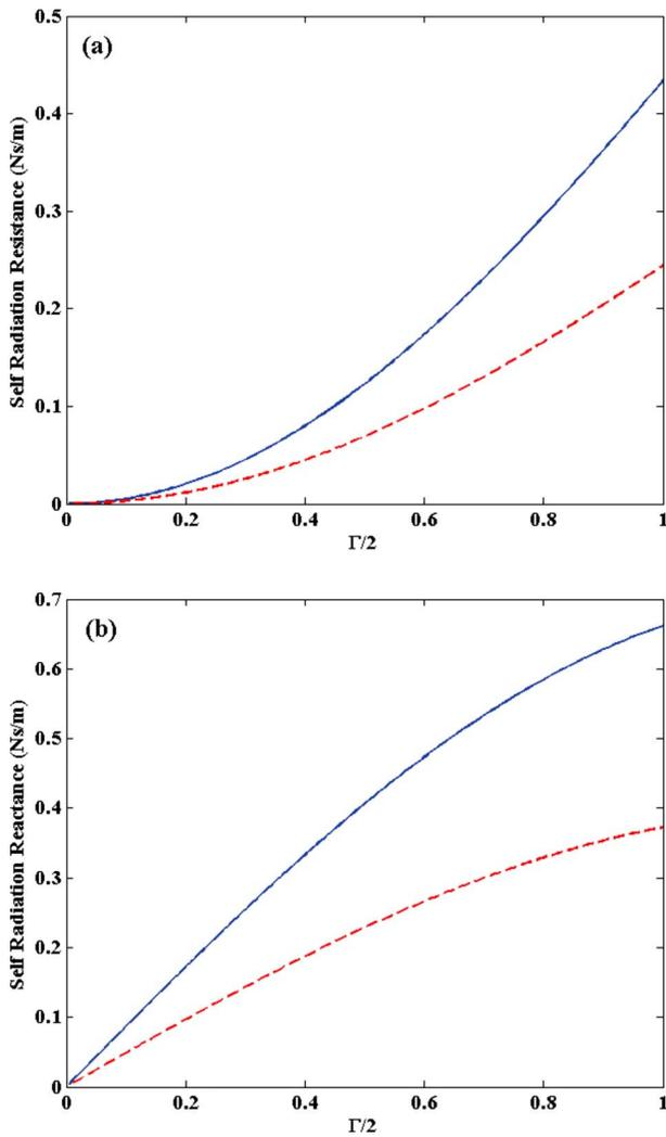
Fig. 5—Effect of number of plate segments (partitions) used on the near field radiation behavior, where  $\Gamma = 2ka_i$ . (a) Self-radiation resistance ( $R_{11}$ ), and (b) self-radiation reactance ( $X_{11}$ ). Key: (blue line) analysis for  $N = 36$  segments, (red dashed line) analysis for  $N = 64$  segments.
