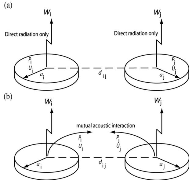
Fig. 2—Illustration of the discrete acoustic models. (a) Without mutual interactions and (b) with mutual interaction between sources (given by  $i$  and  $j$ ).
