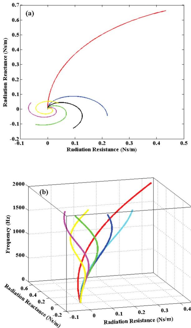
Fig. 7—Comparison of self and mutual radiation impedance terms using the Nyquist diagram. (a) Two dimensional plot, and (b) three dimensional plot. [Key: (red)  $Z_{11}$ , (blue)  $Z_{12}$ , (green)  $Z_{13}$ , (magenta)  $Z_{14}$ , (yellow)  $Z_{15}$ , (black)  $Z_{16}$  calculated for 36 segments and valid for part (a) and (b)].
