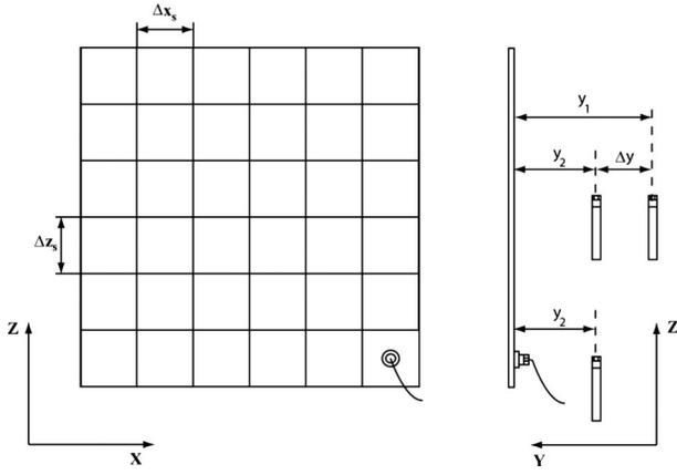
Fig. 3—Schematic of the plate (including discretized elements on the surface) and intensity measurements (using both surface and 2-microphone method). Microphones in the near field along with an accelerometer on the surface are shown in the Cartesian coordinate system.
