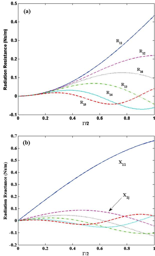
Fig. 4—Effect of self and mutual radiation impedance terms on the near field radiation behavior of the plate, where  $\Gamma = 2ka_i$  and  $j = 2 \dots 6$ . (a) Self ( $R_{11}$ ) and mutual radiation resistance ( $R_{1j}$ ); (b) Self ( $X_{11}$ ) and mutual radiation reactance ( $X_{1j}$ ).
