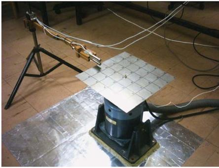
Fig. 1—Example case (free-free steel plate) and near-field acoustic intensity ( $I_m$ ) measurements.
