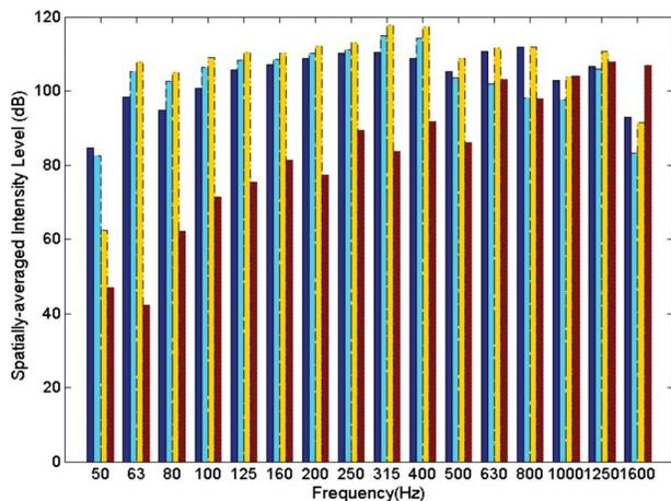
Fig. 10—Contribution of spatially-averaged intensity level  $\bar{I}$ , dB re  $1.0 \text{ pW/m}^2$ , from different regions of the plate on 1/3 octave band basis. Key: Dark blue bars: from the plate center; light blue bars: from the plate corners; yellow bars: from the plate edges (including the corners), red bars: from the top surface of the plate.
