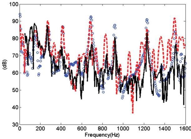
Fig. 8—Measured spatially-averaged intensity ( $\bar{I}$ , dB re  $1.0 \text{ pW/m}^2$ ) and mean-square surface velocity ( $\langle \psi_u^2 \rangle_s$ , dB re  $5.10^{-7} \text{ m/s}$ ), on a narrow band basis. Key: Red dotted line:  $\bar{I}$  by the surface intensity ( $I_s$ ) method; blue circles:  $\bar{I}$  by the two-microphone acoustic intensity ( $I_m$ ) method; black solid line: measured mean-square velocity  $\langle \psi_u^2 \rangle_s$ .
