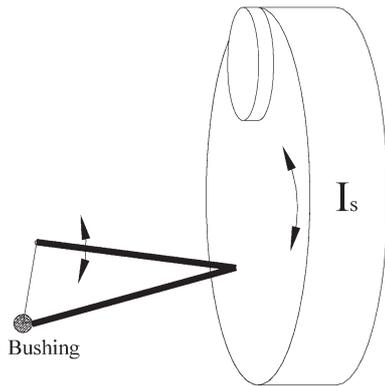
**Fig. 2** Kinematics of the suspension, control arm, and rubber bushing
