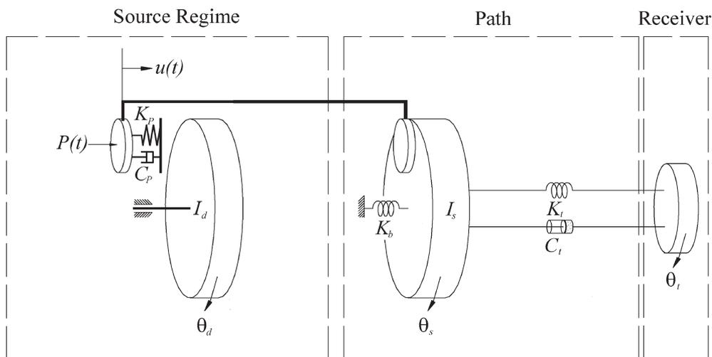
Fig. 1 A simplified source–path–receiver model for brake judder analysis
