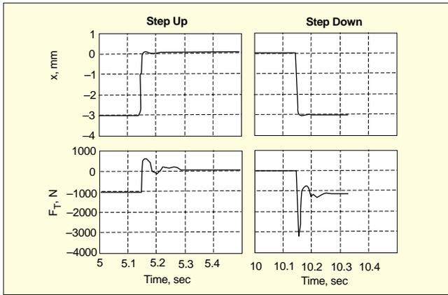
Figure 6. Measured step-up and step-down displacement excitation and transmitted force waveforms for a free decoupler mount.
