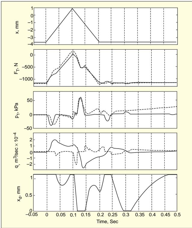
Figure 10. Pulse response of the free decoupler mount (simulations shown as solid plots and measured values shown as dashed plots).
