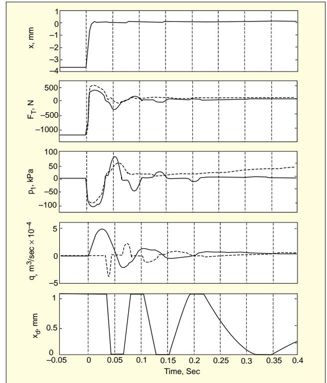
Figure 9. Step response of the free decoupler mount (simulations shown as solid plots and measured values shown as dashed plots).
