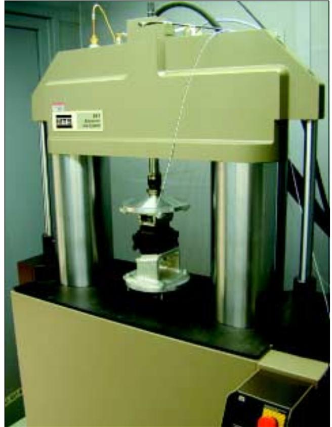
Figure 4. MTS elastomer testing system being used to evaluate the dynamic characteristics of a hydraulic engine mount.
