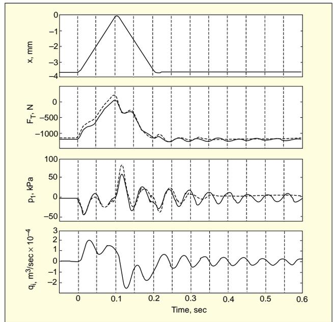
Figure 8. Pulse response of the fixed decoupler mount (simulations shown as solid plots and measured values shown as dashed plots for  $F_T$  and  $p_1$  parameters).
