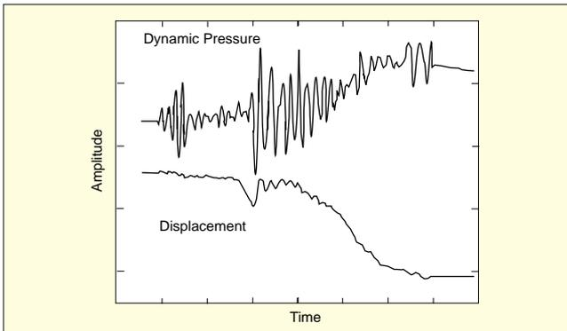
Figure x. Comparison of dynamic pressure response vs. displacement of a hydraulic engine mount.
