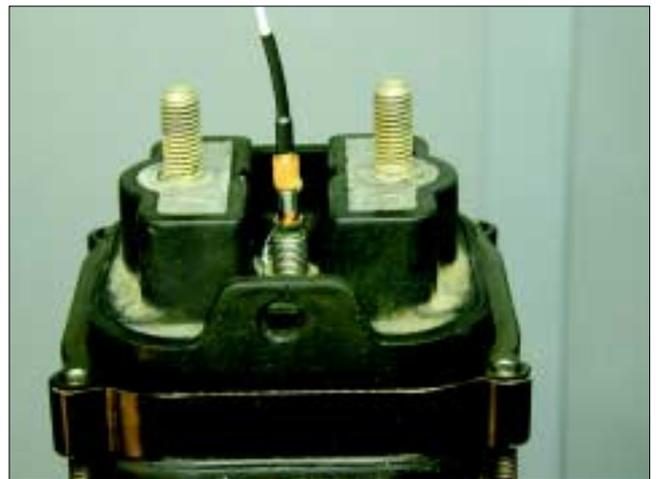
Figure 5. Dynamic pressure transducer installed in the top chamber of a hydraulic engine mount.
